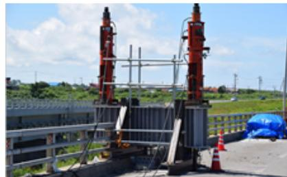
Figure 2. Loading device.
