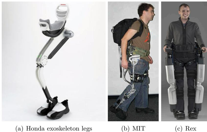
Figure 1.2: Power assist robots designed for elderly/disabled support
