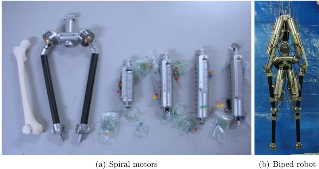
Figure 6.6: Biped robot with bi-articular actuation realized using spiral motors [27] [112]
