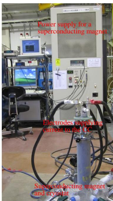
Figure 2-9: Equipment to apply external magnetic field and electrodes supplying current to the CC.
