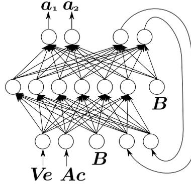
Figure 3.8: RNN used in the experiment.  $Ve$ : Velocity of a hand,  $Ac$ : Acceleration of a hand,  $a_1, a_2$ : Outputs to calculate  $A_1, A_2$  in Equation 3.5, respectively,  $B$ : Bias neuron
