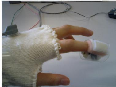
Figure 3.6: The sensor and the ICPF tactile display on a hand
