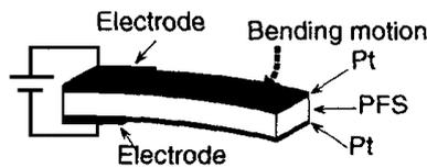
Figure 3.4: ICPF actuator (from Konyo et al. (Konyo et al., 2000))
