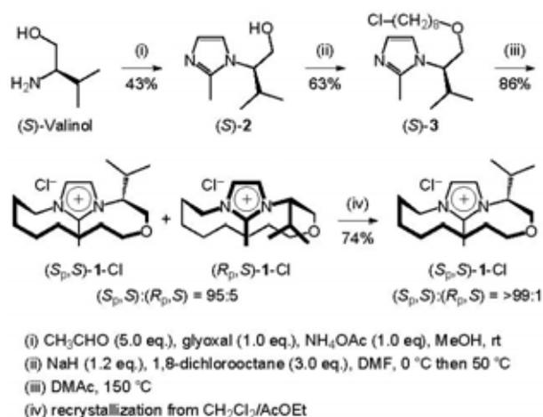
**Scheme 1.** Synthesis of the planar-chiral imidazolium salt **1-Cl**
