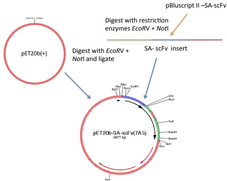
**Figure 4-4.** Cloning to make pET20b+SA-scFv plasmid.
