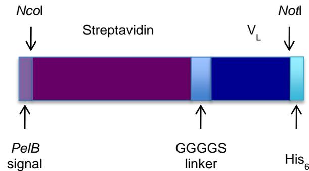
**Figure 3-2.** Construction of SA-V<sub>L</sub> expression vector. The construct was made by PCR, and inserted to pET20b+ vector plasmid.
