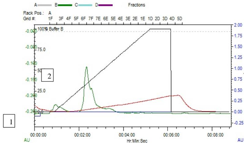
**Figure 3-4.** Anion-exchange chromatography of SA-V<sub>L</sub> protein purification by using (25 mM Tris-HCl, pH 8.1) as an equilibrium buffer and (25 mM Tris-HCl with 0.5 M NaCl, pH 8.1) is used as elution buffer to elute purified SA-V<sub>L</sub> protein from column of an Uno-Q1 column on a Biologic Duo-Flow system (Bio-Rad). Here, peak 1 is non-related protein and peak 2 is SA-V<sub>L</sub> protein as it is confirmed by SDS-PAGE experiment.
