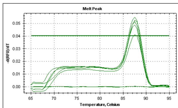
**Figure 3-11.** Melt peaks for streptavidin-based OS Immuno-PCR. The peak of dissociation curves shows the melting temperature.
