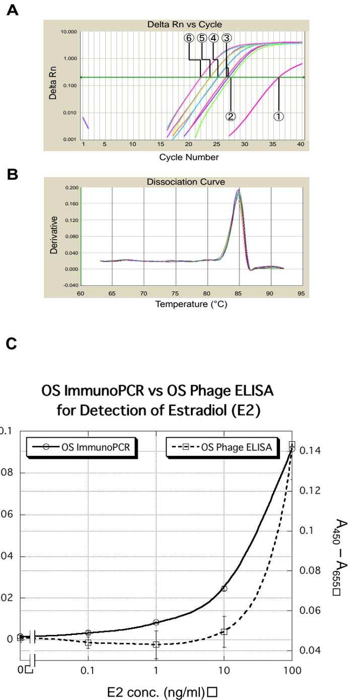
**Figure 2-5.** (A) Result for quantitative PCR for E2 quantification. (1) Without MBP-V<sub>L</sub> immobilization; (2) E2 concentration of 0 ng/ml; (3) 0.1 ng/ml; (4) 1 ng/ml; (5) 10 ng/ml; (6) 100 ng/ml. Two overlapping curves for each E2 concentration are shown. (B) Dissociation curves showing the melting temperature. (C) Comparison of dose–responses for OS phage Immuno-PCR and OS phage ELISA. Average values  $\pm$  1 SD are shown (n = 2).
