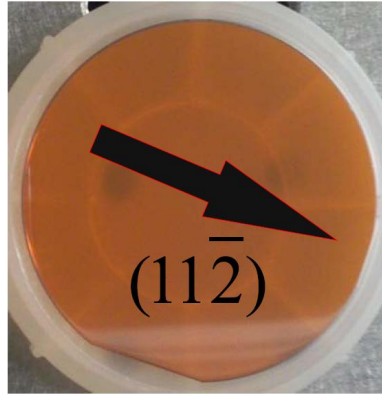
Figure 5.8: A wafer of high resistance GaP(111) crystal - the thickness of the wafer is 50\mu\text{m} , and the diameter of the wafer is 2 inches.
