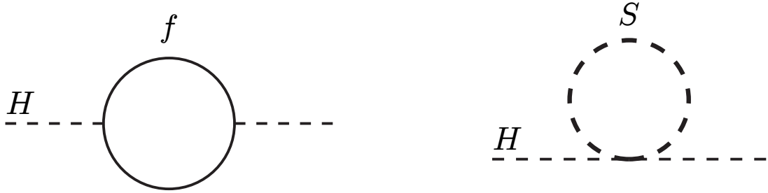
Figure 3: Example diagrams showing 1-loop radiative corrections which contribute to m_h . The loop of a Dirac fermion f (left) with a coupling constant \lambda_f and the one of a scalar particle S (right) with a coupling constant \lambda_S .
