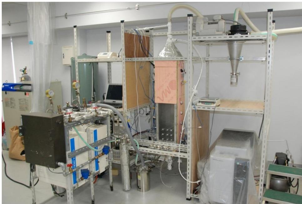
**Fig. 3-2-2.** Schematic diagram of an experimental fluidized bed dryer
