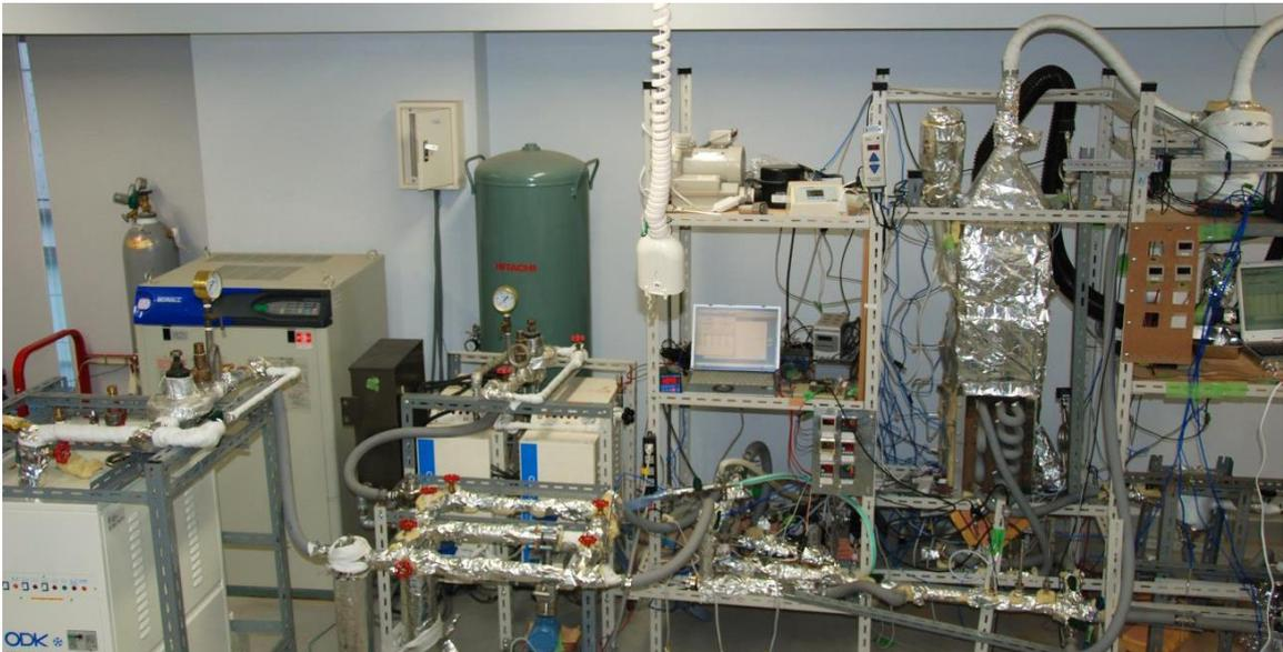
**Fig. 5-3-1.** Schematic diagram of an experimental fluidized bed dryer
