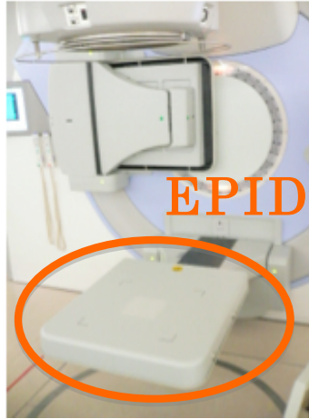
Fig. 2-1: An electronic portal imaging device (EPID) mounted on the linear accelerator (LINAC) (Elekta). The detector panel is a PerkinElmer Amorphous Silicon (a-Si) detector, and provides a resolution of 1024 \times 1024 16-bit pixel images, with a detector panel size of 41 \times 41 cm (approximately 26 \times 26 cm at isocenter). Image data is read from the panel, through a data link into a framegrabber in the iViewGT™ (Elekta).
