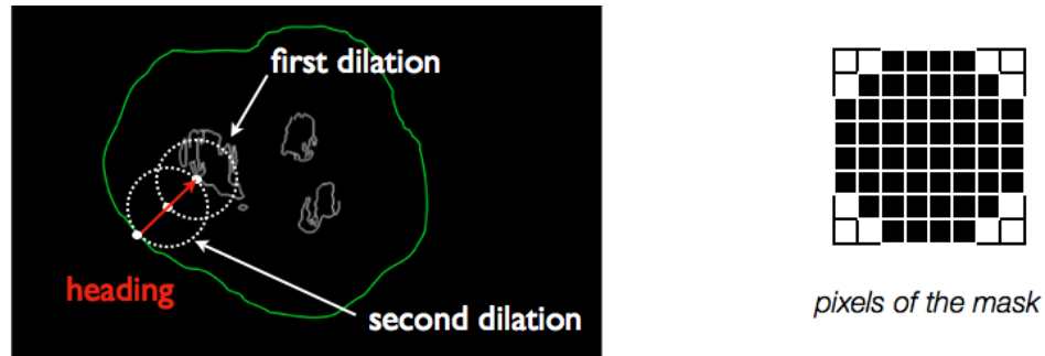
Fig. 4.18. Performing observations around rocks without landing; Green: Scanning path identified by image processing, Red: Scanning heading to face the target
