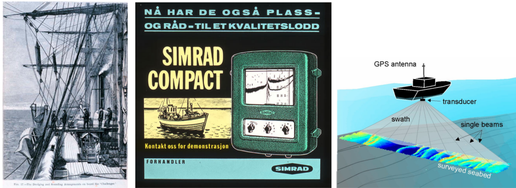
Fig. 1.2. Instruments for scanning the seafloor; Left: HMS Challenger survey Source: NOAA Photo Library , Centre: Simrad echo sounder Source: Kongsberg Maritime AS , Right: Multi-beam swath sounding sonar Source: Qyudos Geosurvey
