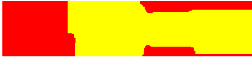
Fig. 4.9. Detected flat area where the vehicle of a particular size can fit. Red: unsafe area with features, Yellow: flat area where vehicle can fit
