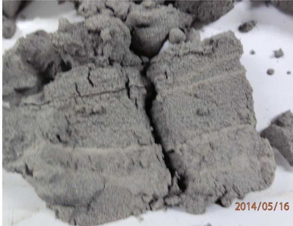
**Figure 5.63. Layering observed in samples made by SD**
