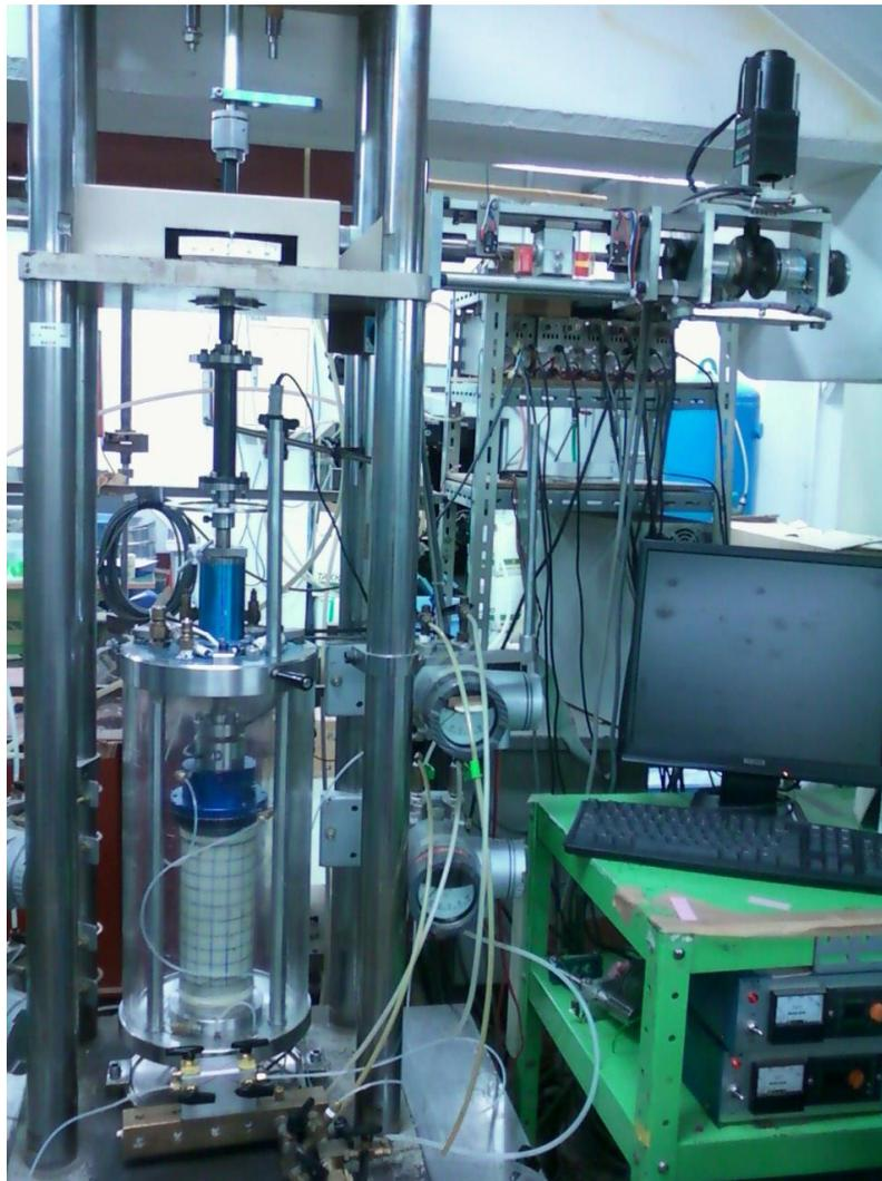
**Figure 4.6. Hollow cylinder torsional shear device**
