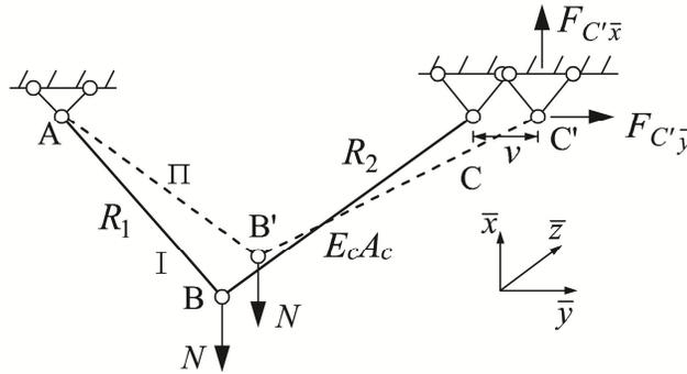
Fig.6-4 Mechanistic movements of cables in-plane
