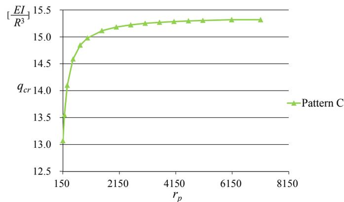
(b)  $r_p \in [153.36, 7156.62]$ Fig.5-16 Relationship of  $r_p$  and first order critical load  $q_{cr}$  (hinged ended)
