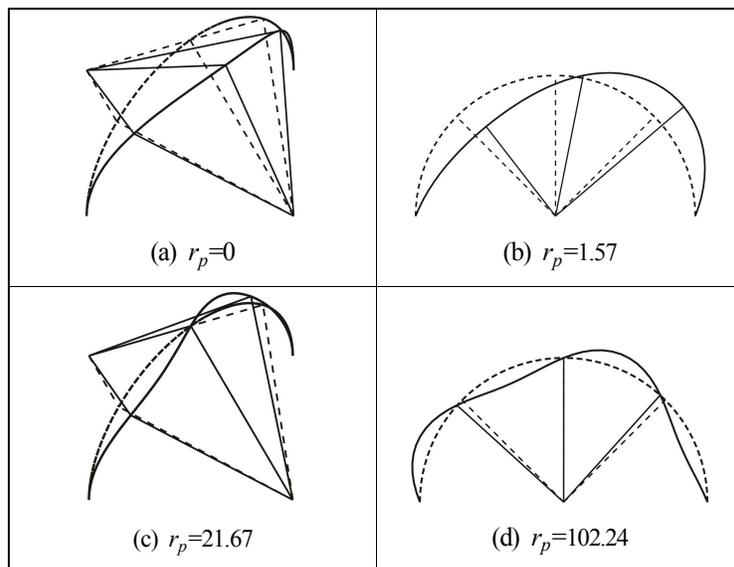
Table.5-8 shows the final first order buckling modes of all stiffening patterns, which are corresponding to the first order critical loads in Fig.5-20. When  $r_p$  is very large, we can observe that the first order buckling modes of Pattern D and Pattern DE happen in-plane, while the one of Pattern E happens out-of-plane.
