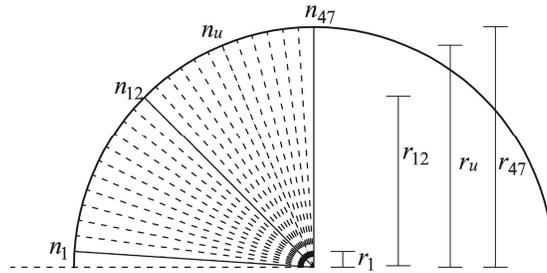
Fig.D-2 Heights of nodes in the circular arch
