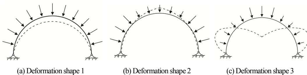
Fig.2-2 Three types of deformations
