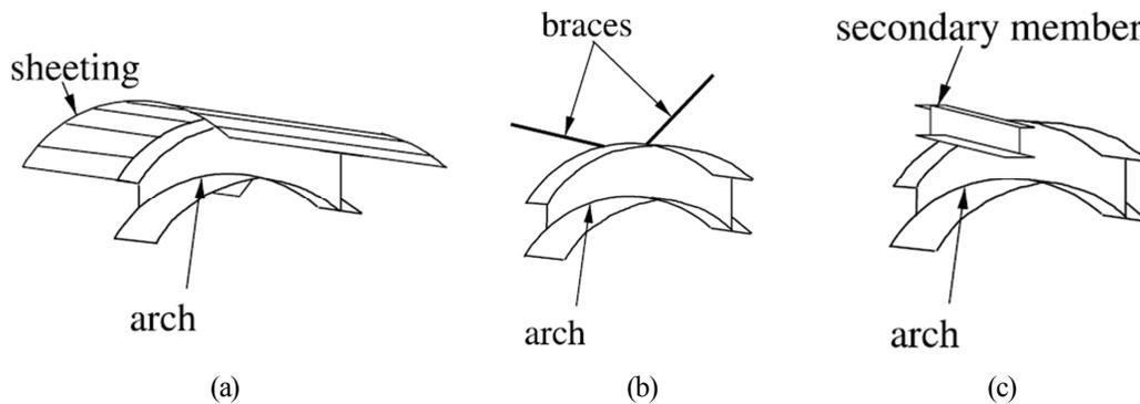
Fig.1-1 Constraint components at local places of the arch structures<sup>[144]</sup>
