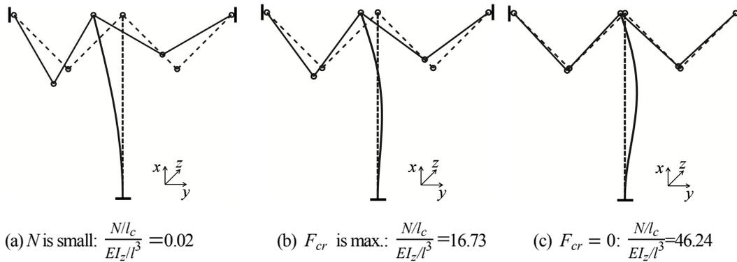
Fig.6-13 First order buckling modes in-plane by FE method
