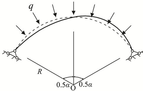
Fig.4-5 Buckling of the arch in-plane
