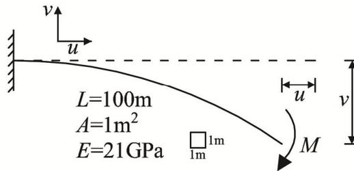
Fig.3-6 Cantilever beam under bending moment<sup>[159]</sup>
