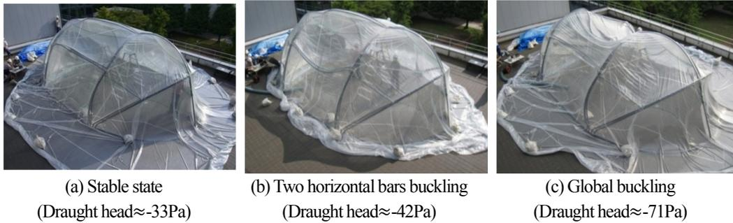
Fig.7-21 Deflating experiment in May
