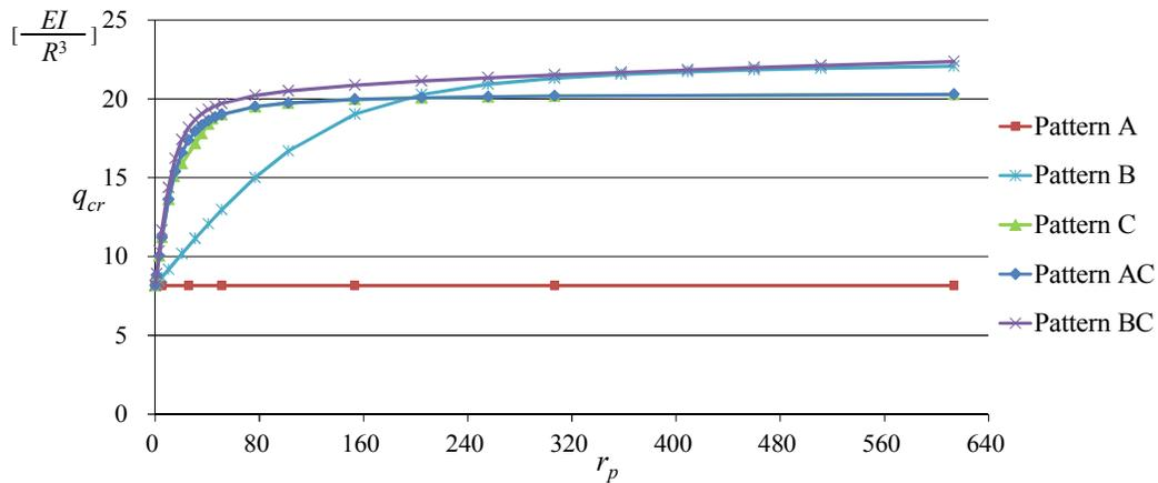
Fig.5-17 Relationship of  $r_p$  and first order critical load  $q_{cr}$  (fixed ended)
