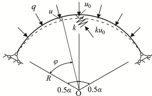
Fig.E-2 Arch-spring model out-of-plane
