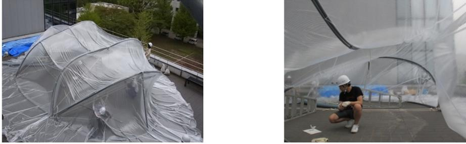
Fig.7-18 Buckling of skeletons of rectangle shelter in April ( $\approx -30\text{Pa}$ )
