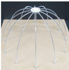
Fig.7-1 Miniature model of hemispheric shelter
