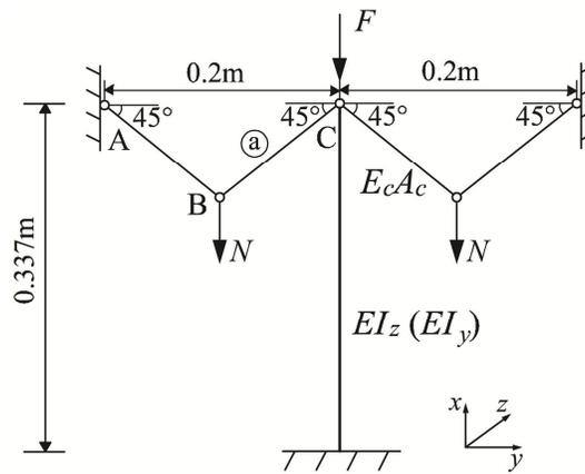
Fig.6-8 Column featuring with curved cables
