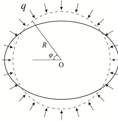
Fig.5-33 Buckling problem of ring in-plane
