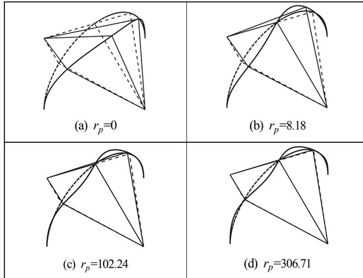
Table.5-10 shows the final first order buckling modes of all stiffening patterns. When  $r_p$  is very large, the first order buckling modes of Pattern D, Pattern E and Pattern DE all happen out-of-plane.
