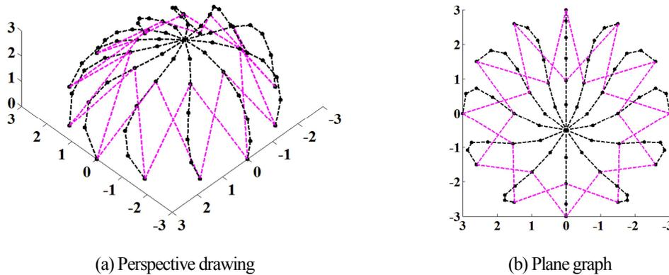
Fig.7-13 First order buckling mode with ropes (First order critical load= $-25.2\text{Pa}$ )
