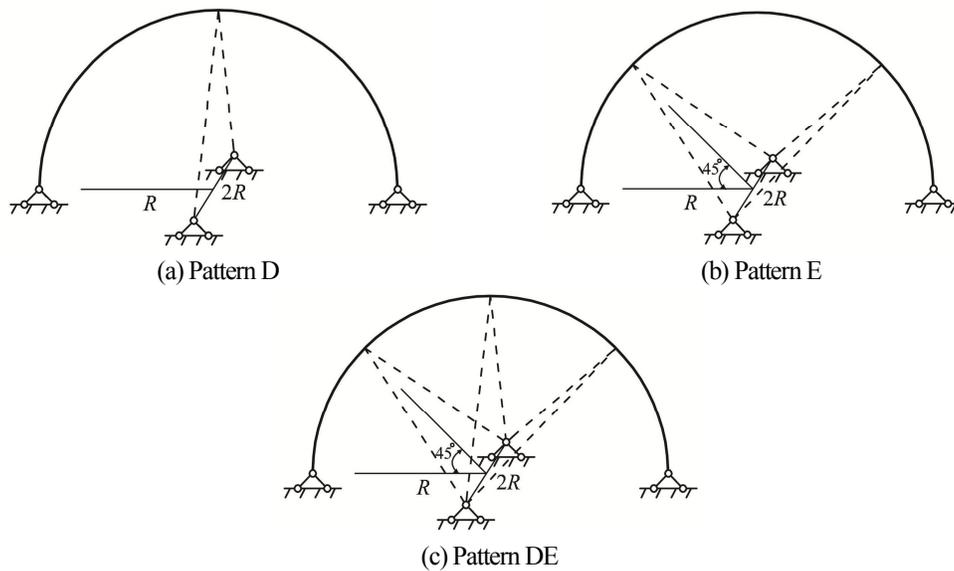
Fig.E-4 Stiffening patterns of single arch out-of-plane
