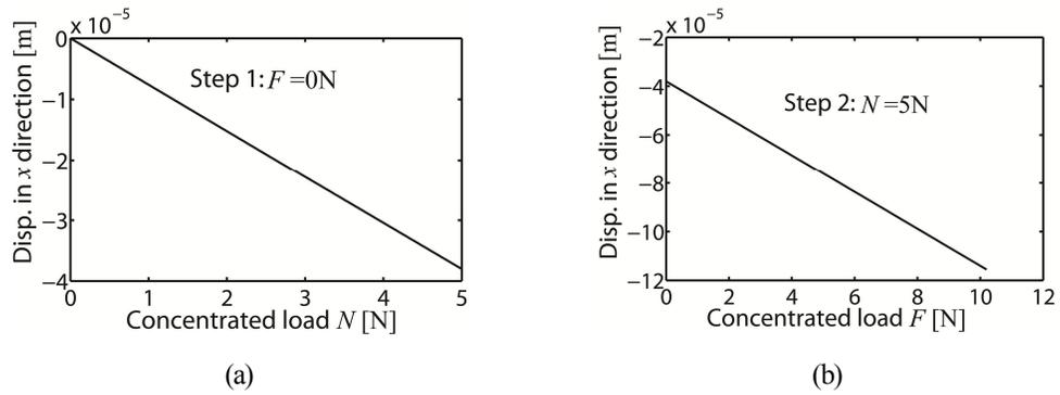
Fig.6-10 Relationship of displacement with  $N$  and  $F$
