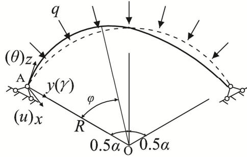
Fig.4-10 Buckling of the arch out-of-plane
