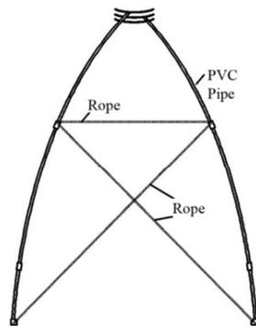
Fig.7-5 Setting of stiffening rope
