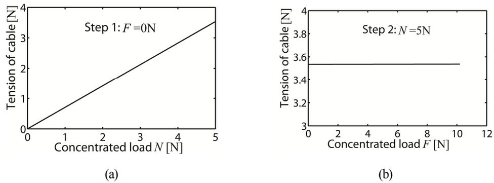
Fig.6-11 Relationship of tension of cable with  $N$  and  $F$
