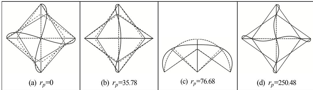
Table.5-12 shows the final first order buckling modes of call stiffening patterns. And Pattern F and Pattern G have the same buckling modes. The buckling modes of Pattern H, Pattern FH and Pattern GH are almost identical.
