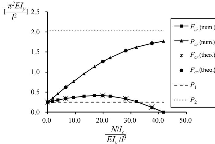
Fig.6-15 Relationship of  $\frac{N/l_c}{EI_y/l^3}$ ,  $F_{cr}$  and  $P_{cr}$  out-of-plane
