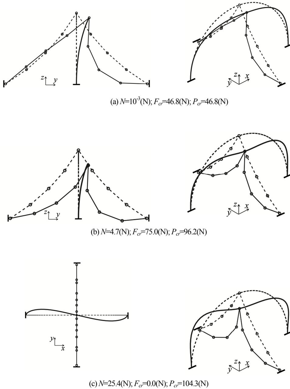
Fig.6-26 First order buckling modes of the arch with curved cables
