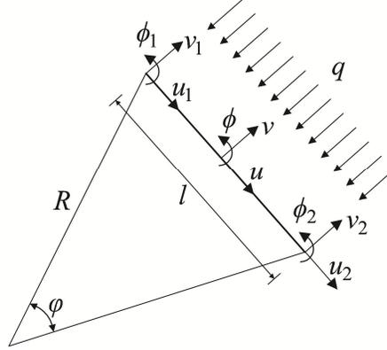
Fig.3-4 A straight beam element for the circular arch/ring <sup>[74]</sup>
