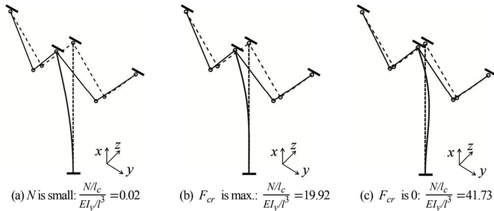
Fig.6-16 First order buckling modes out-of-plane by n FE method
