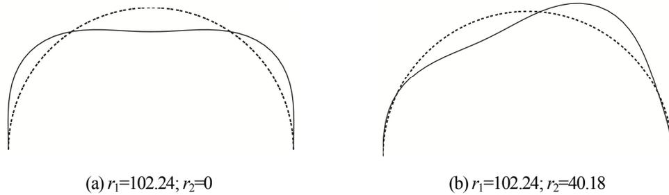
Fig.5-9 First order buckling modes ( $r_1=102.24$ )
