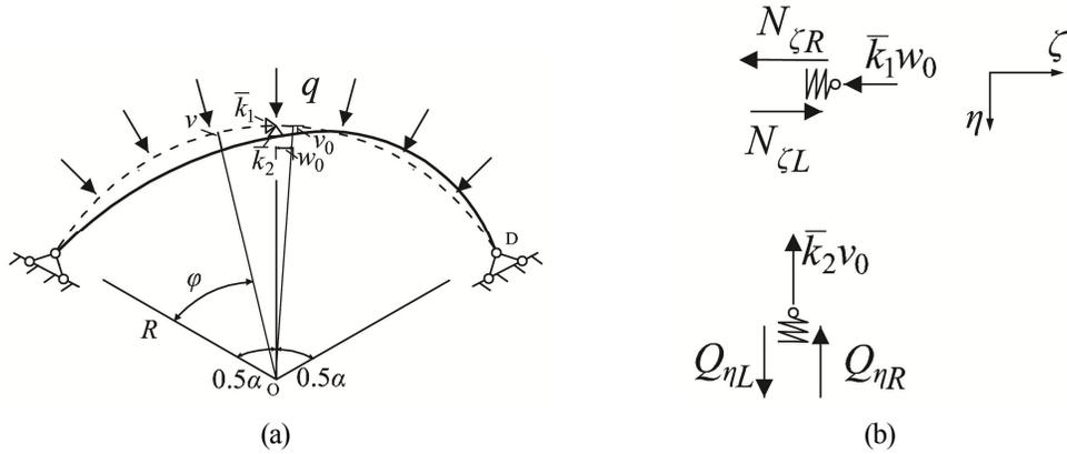
Fig.5-3 Circular arch stiffened by two springs
