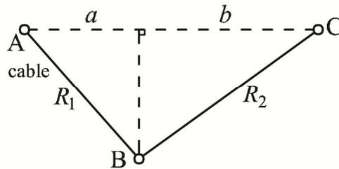
Fig.6-6 Initial geometric shape of curved cables
