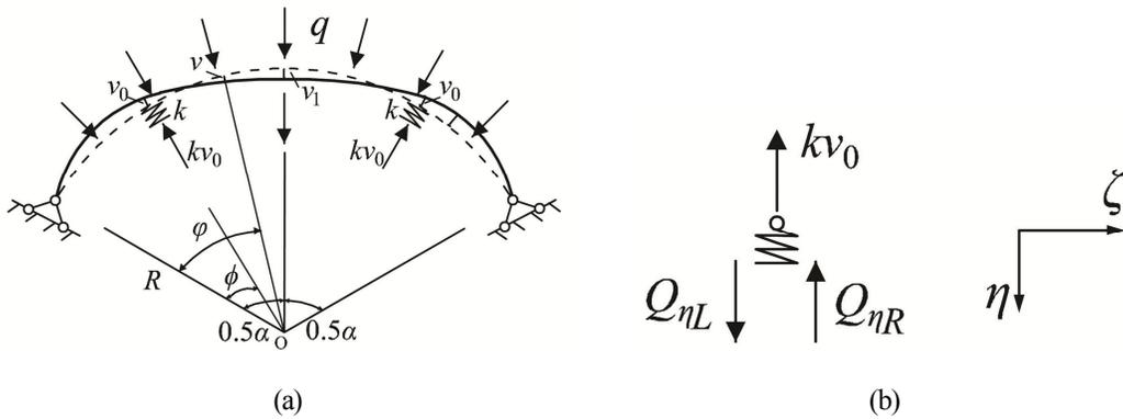
Fig.B-3 Circular arch with hinged ended boundary conditions
