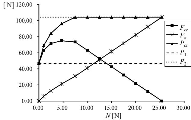
Fig.6-24 Relationship of the concentrated load on cables and the critical load
