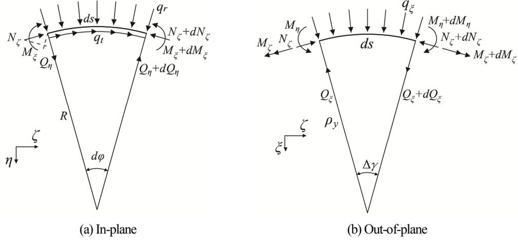
Fig.B-5 Isolated infinitesimal body of the arch (in Chapter 4) <sup>[108]</sup>
