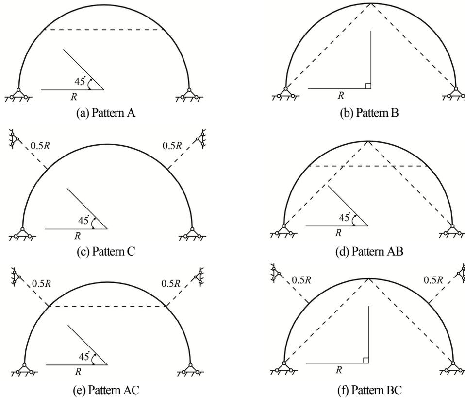
Fig.E-3 Stiffening patterns of single arch in-plane
