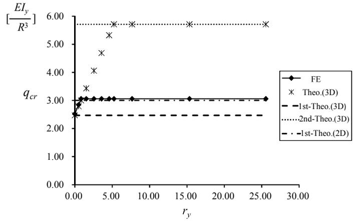
Fig.5-12 Relationship of  $r_y$  and  $q_{cr}$  with hinged ended boundaries in-plane
