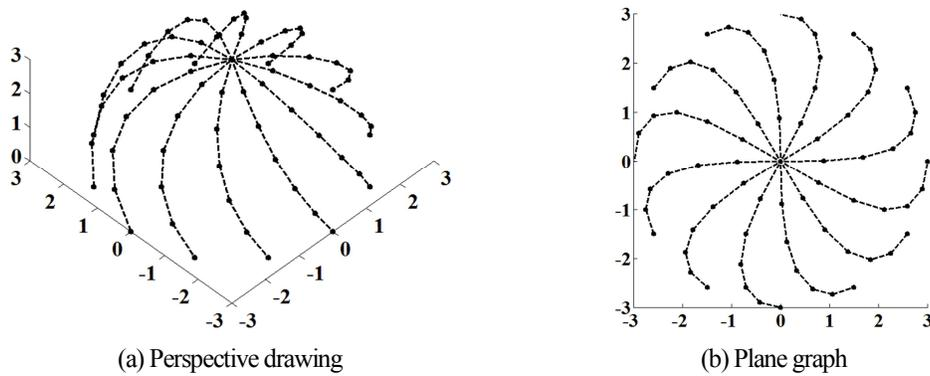
Fig.7-11 First order buckling mode without ropes (First order critical load=8.6Pa)
