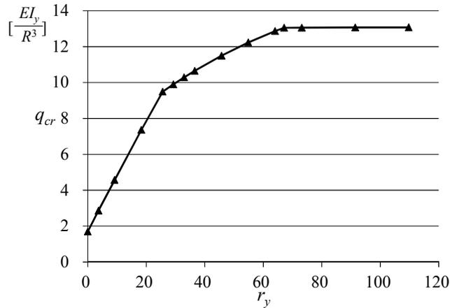
Fig.5-35 Relationship of parameter  $r_y$  and the first order critical load  $q_{cr}$
