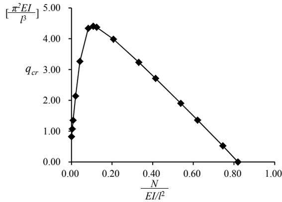
Fig.6-19 Relationship of  $\frac{N}{EI/l^2}$  and critical distributed load  $q_{cr}$
