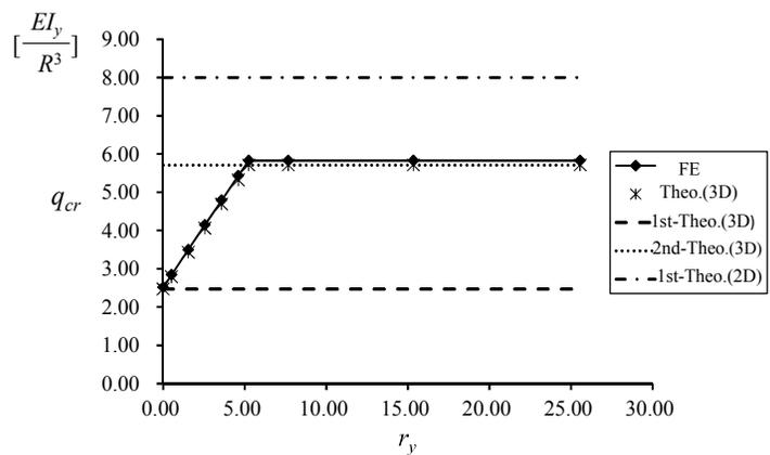
Fig.5-13 Relationship of  $r_y$  and  $q_{cr}$  with fixed ended boundaries in-plane
