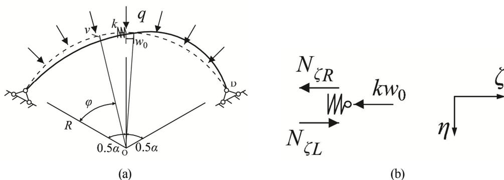
Fig.5-1 Anti-symmetric arch-spring model
