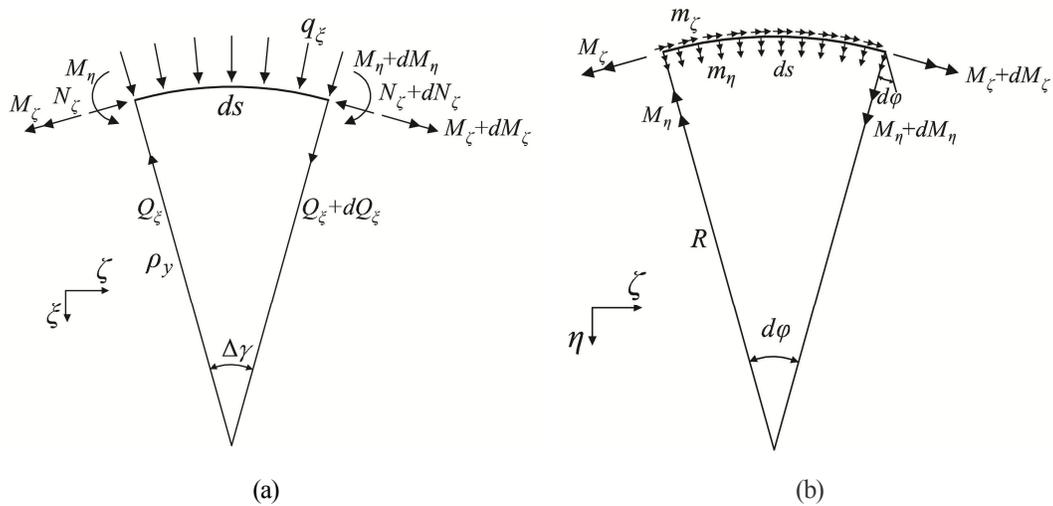
Fig. 4-7 Equilibrium state of forces out-of-plane<sup>[108]</sup>
