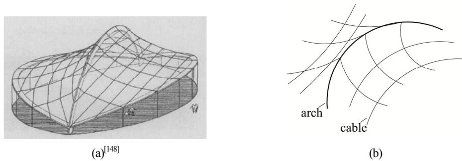
Fig.1-4 Arch structures supported by cable-nets
