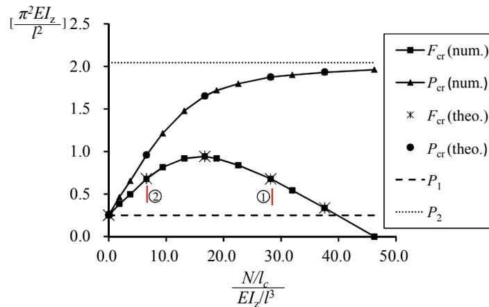
Fig.6-12 Relationship of  $\frac{N/l_c}{EI_z/l^3}$ ,  $F_{cr}$  and  $P_{cr}$  in-plane
