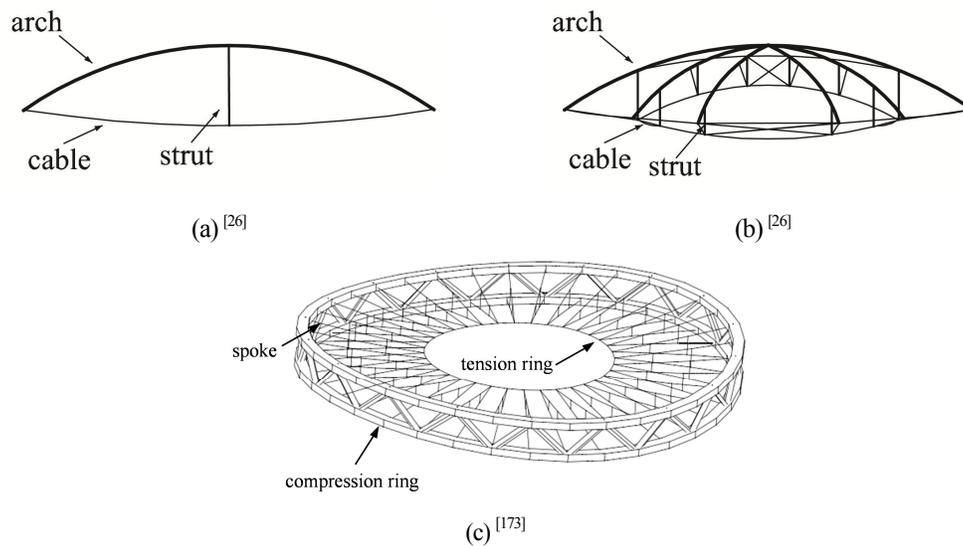
Fig.1-3 Arch with components at boundary
