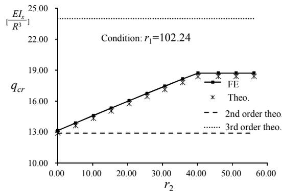
Fig.5-8 Comparison of the results with fixed ended boundaries
