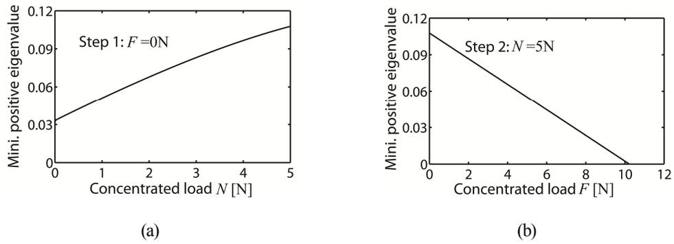
Fig.6-9 Relationship of minimum positive eigenvalue with  $N$  and  $F$
