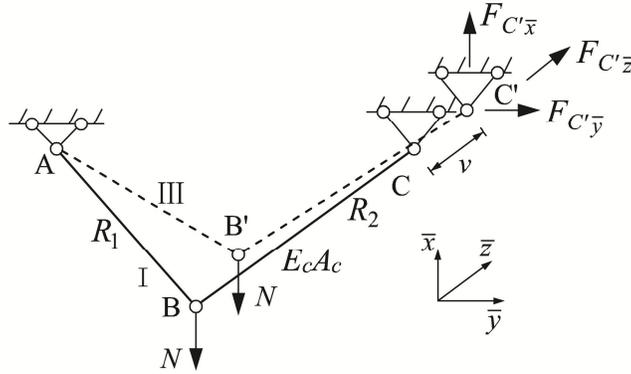
Fig.6-5 Mechanistic movements of curved cables out-of-plane
