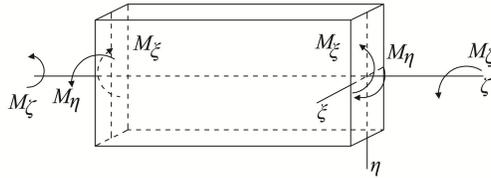
Fig.4-3 Moments in the isolated infinitesimal body<sup>[108]</sup>
