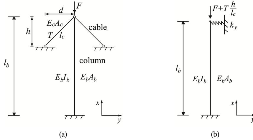
Fig.6-2 Column stiffened by straight cables
