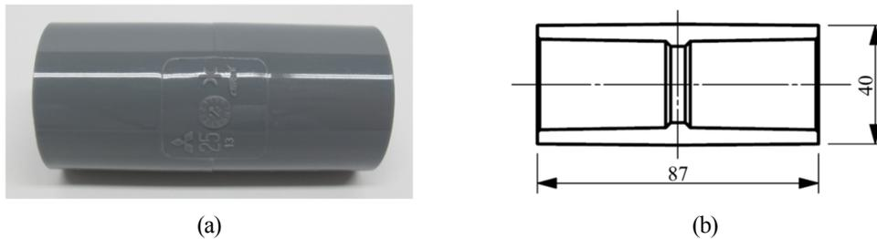
Fig.7-4 Joint of PVC pipes
