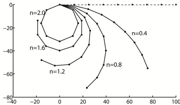
Fig.3-7 Shape of cantilever after deformation
