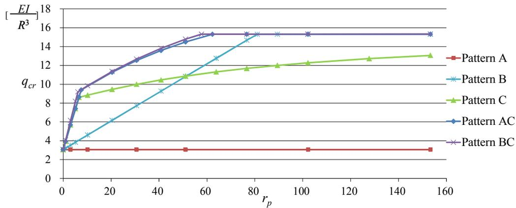
(a)  $r_p \in [0, 153.36]$
