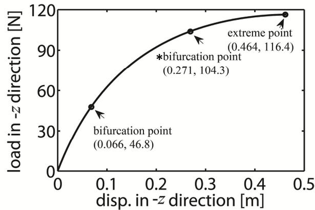
Fig.6-23 The relationship of displacement and load in  $-z$  direction
