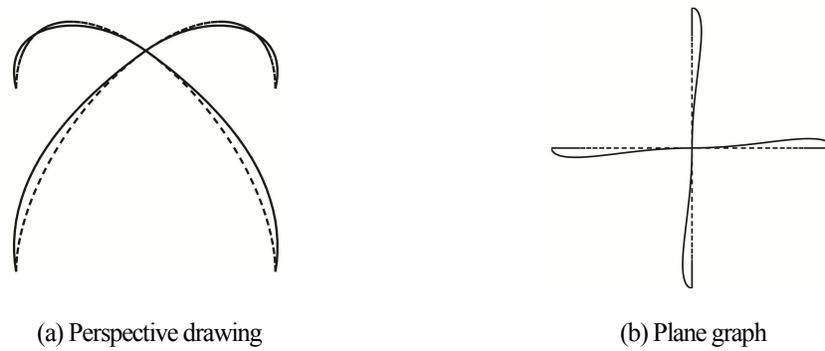
Fig.5-26 Third order buckling mode of cross arch
