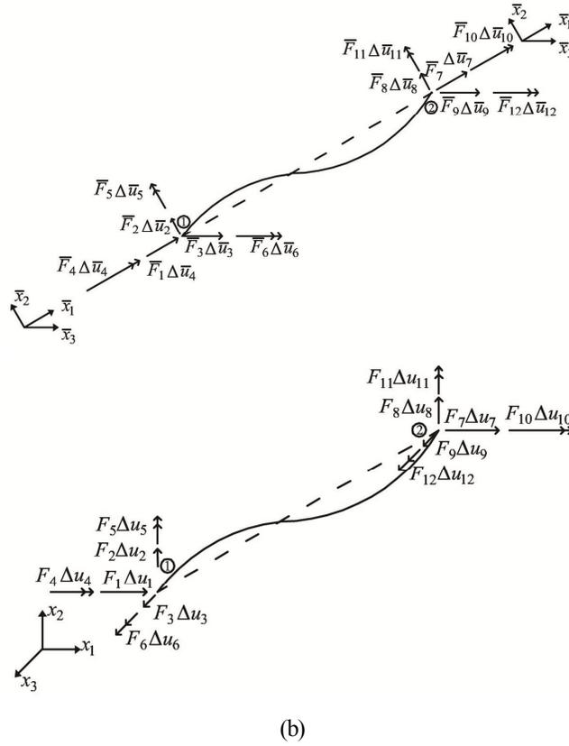
Fig.3-2 Displacements and internal forces of beam element<sup>[86],[101]</sup>
