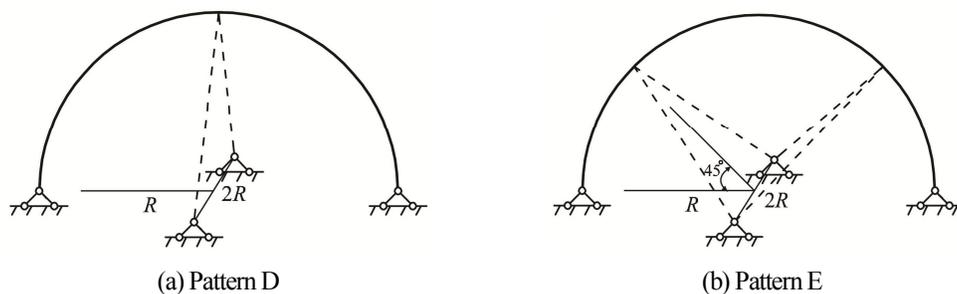
Fig.5-18 Two basic stiffening patterns out-of-plane
