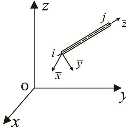
Fig.3-1 Global and local Cartesian coordinate system of 3D-beam element
