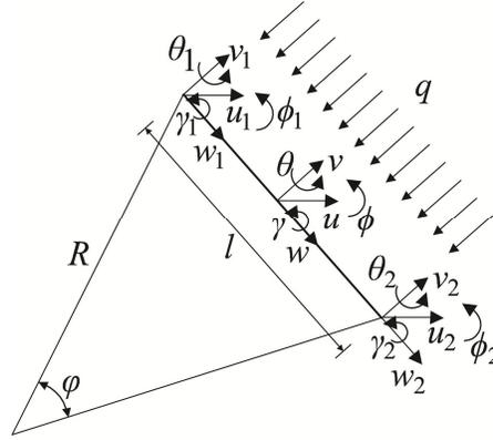
Fig.3-5 A straight beam element for a circular arch/ring
