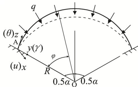
Fig.4-11 Buckling of the arch out-of-plane
