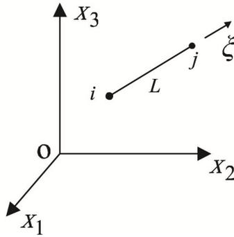
Fig.3-3 Truss element in 3D space <sup>[151]</sup>
