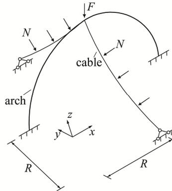
Fig.6-21 Arch featuring with curved cables
