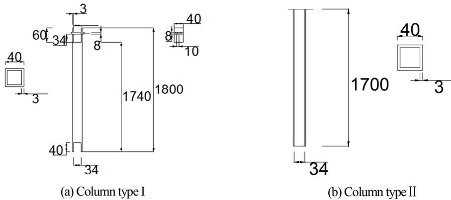
Fig.7-24 Two types of columns
