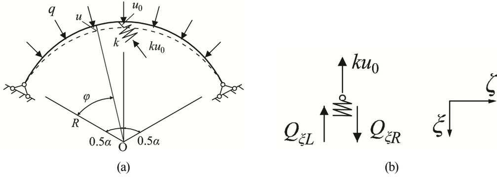
Fig.5-11 Arch-spring model out-of-plane
