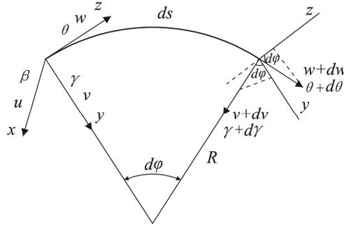
Fig.4-2 Displacements in the isolated infinitesimal body of the arch <sup>[108]</sup>
