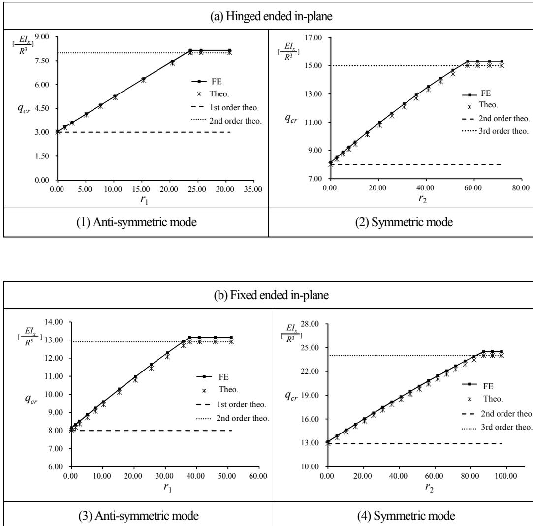
In another aspect, from Table.5-1 it is straightforward to observe that in these four configurations, the theoretical results are almost in accordance with the ones obtained by FE method. The small differences exist because of the different division numbers of beam elements in FE methods. And the higher division number of elements is, the higher accuracy of FE results becomes.
