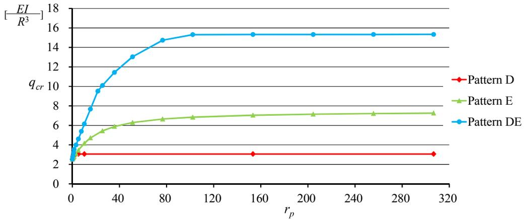
Fig.5-20 Relationship of  $r_p$  and first order critical load  $q_{cr}$
