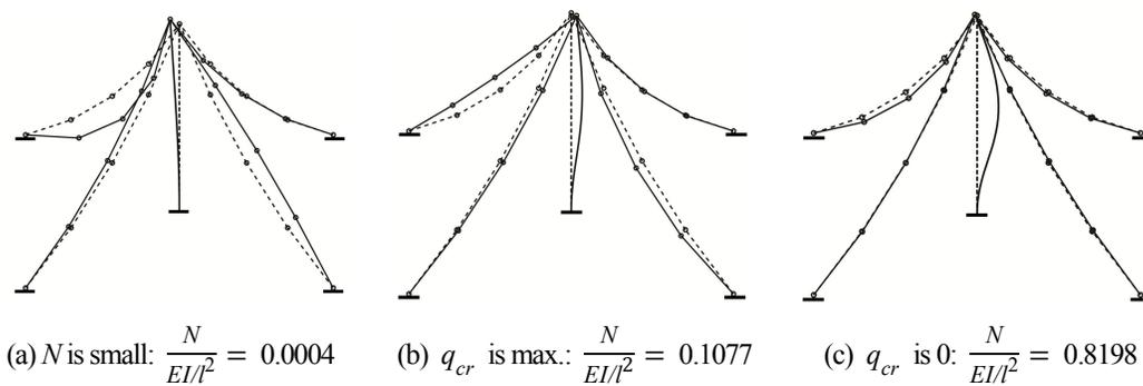
Fig.6-20 First order buckling modes by FE method
