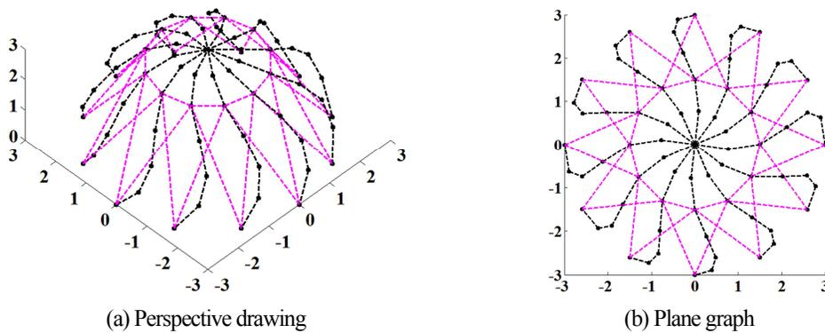
Fig.7-12 First order buckling mode with ropes (First order critical load=44.0Pa)
