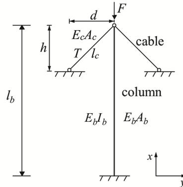
Fig.C-1 Column stiffened by straight cables <sup>[174]</sup>
