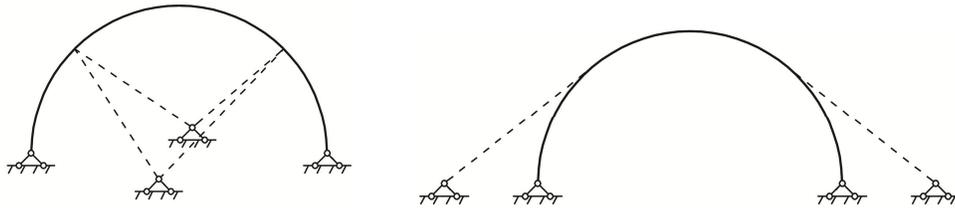
Fig.2-5 External reaction type of single arch
