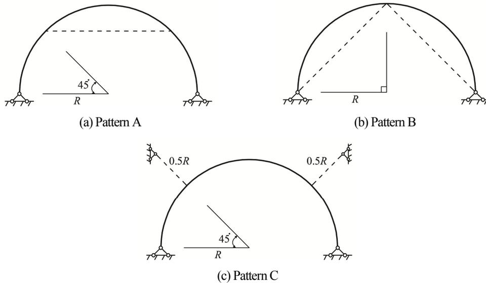
Fig.5-14 Three basic stiffening patterns in-plane
