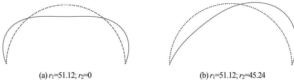
Fig.5-6 First order buckling modes ( $r_1=51.12$ )
