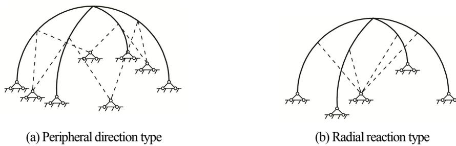
Fig.2-8 External reaction type of cross arch
