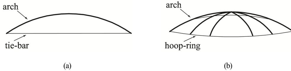
Fig.1-2 Arches with components in the boundary<sup>[26]</sup>
