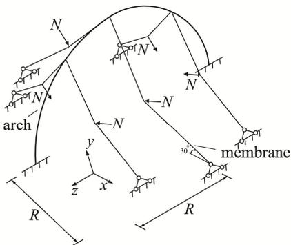
Fig.7-32 Model of the arch
