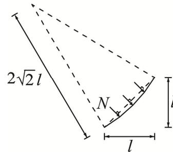
Fig.6-18 Shape of curved cables
