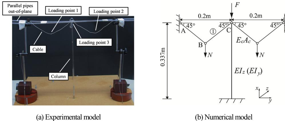
Fig.7-37 Experimental model and numerical model
