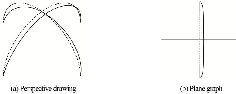
Fig.5-25 Second order buckling mode of cross arch
