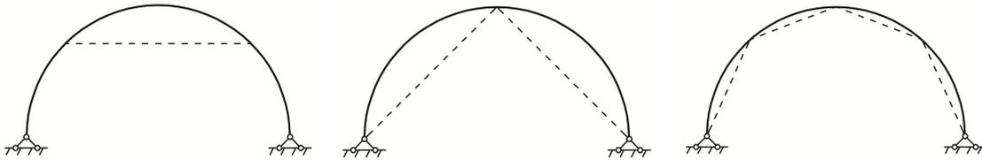
Fig.2-3 Longitudinal direction type/Internal reaction type of single arch
