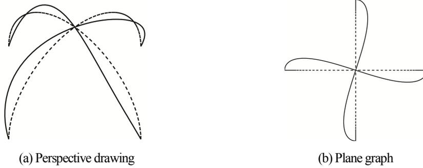
Fig.5-24 First order buckling mode of cross arch
