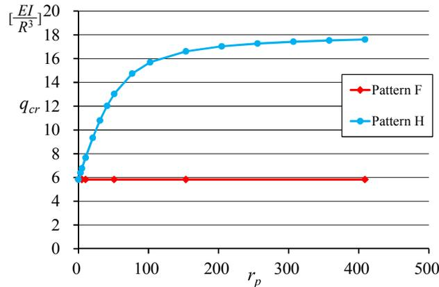
Fig.5-31 Relationship of  $r_p$  and the first order critical load  $q_{cr}$  ( fixed ended boundaries)
