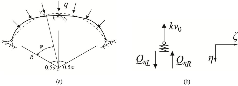
Fig.5-2 Symmetric arch-spring model
