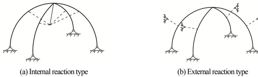
Fig.2-7 Radial direction type of cross arch
