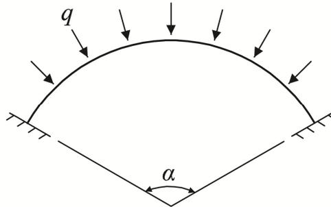
Fig.4-1 Circular arch under uniform compression
