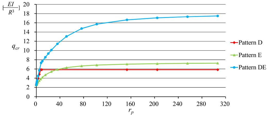
Fig.5-21 Relationship of  $r_p$  and first order critical loads  $q_{cr}$
