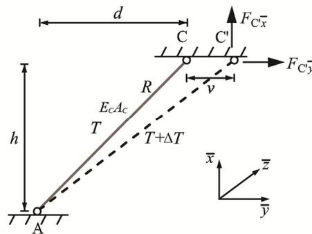
Fig.C-2 Movement of straight cable
