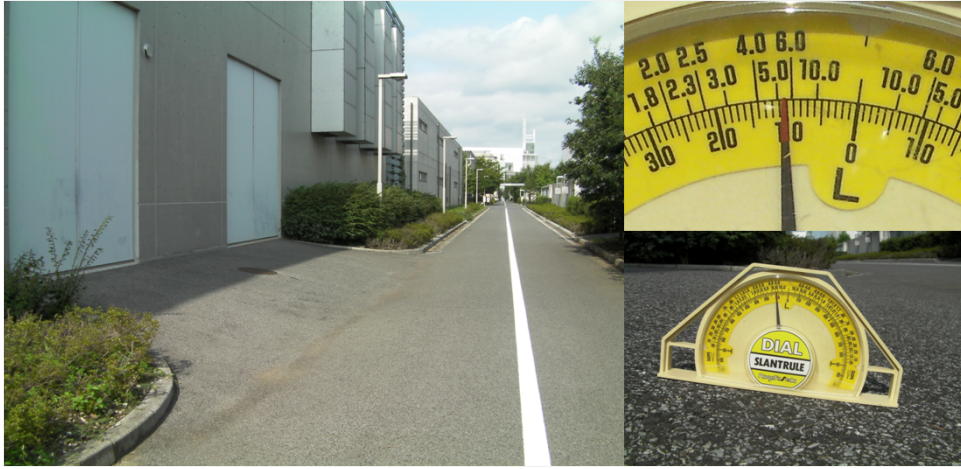
Figure 2.17: Bank where the experiment was carried out. The bank angle is 10.5 degrees.
