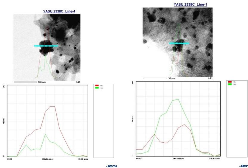
**Fig. 1-2-5. Line analyses of PI/CB Rh/Ag IV-2**
