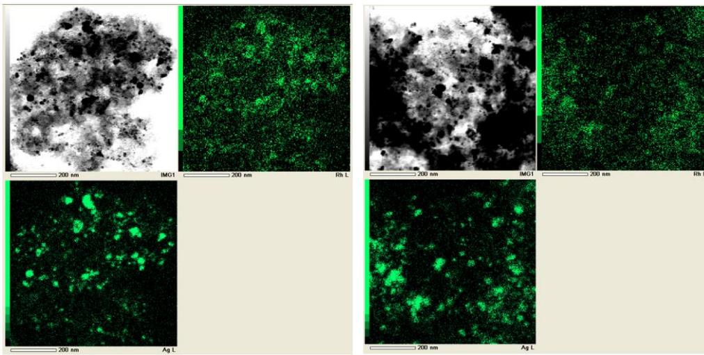
Fig. 1-2-13. EDS analyses of PI/CB Rh/Ag IV-5
