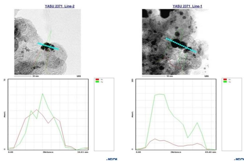
**Fig 1-2-11.** Line analyses of PI/CB Rh/Ag IV-4
