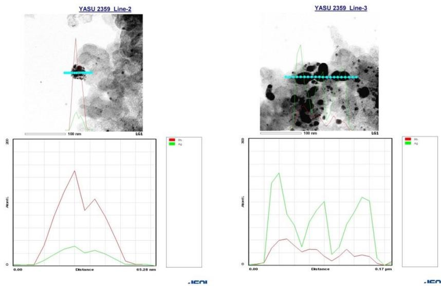
**Fig. 1-2-8. Line analyses of PI/CB Rh/Ag IV-3**
