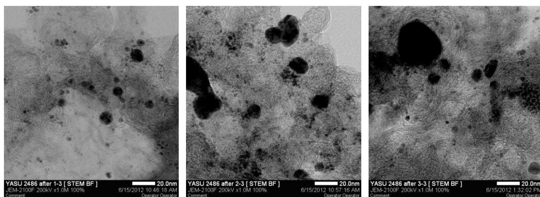
**Fig. 1-2-23.** STEM images of PI/CB Rh/Ag IV-2 (after 10th use and heating)
