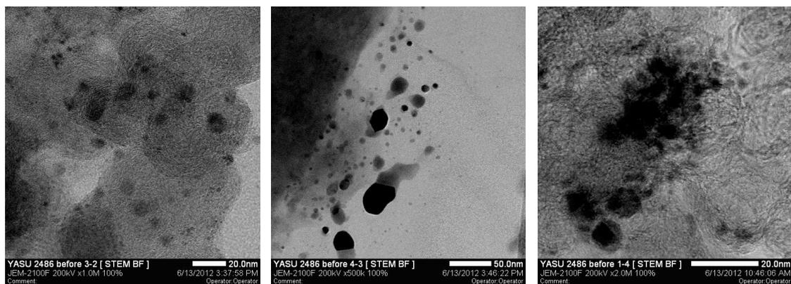
**Fig. 1-2-21.** STEM images of PI/CB Rh/Ag IV-2 (after 10th use, before heating)
