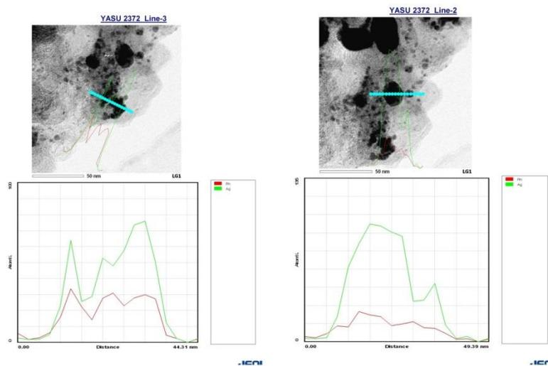
Fig 1-2-14. Line analyses of PI/CB Rh/Ag IV-5
