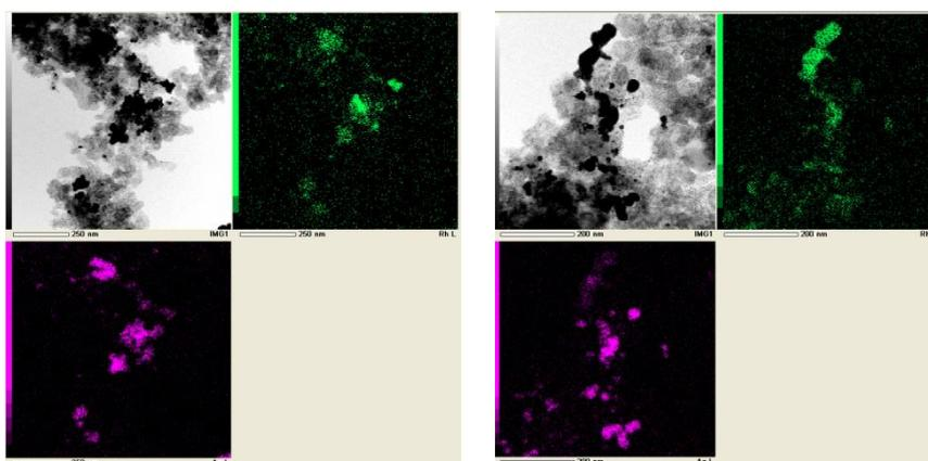
Fig. 1-2-19. EDS analyses of PI/CB Rh/Ag IV-6
