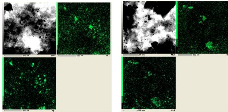
**Fig. 1-2-4. EDS analyses of PI/CB Rh/Ag IV-2**
