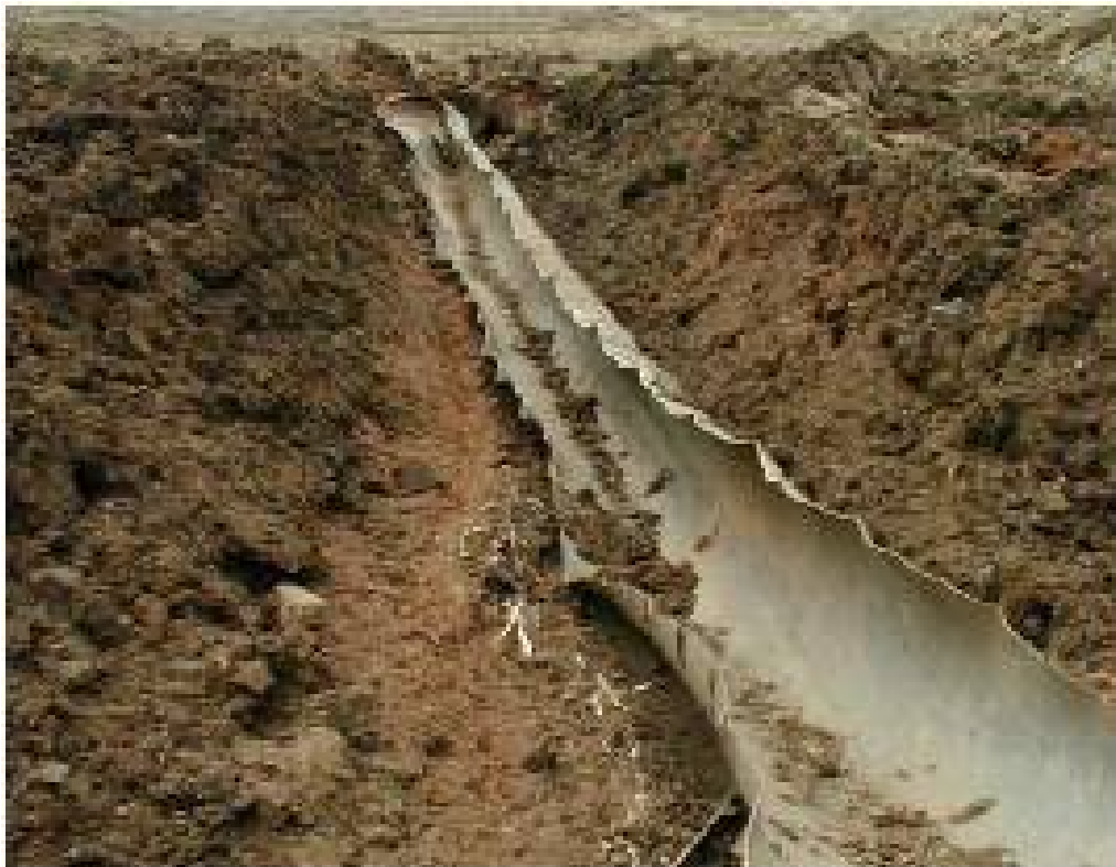
Fig. 1.13 Photo of unstable ductile crack propagation[16]
