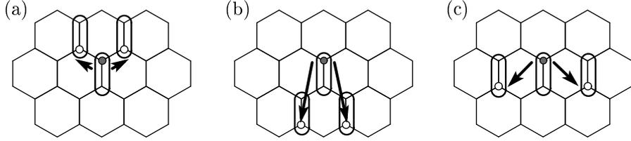
Fig. 2.  $L \rightarrow R$  hoppings to nearest unit cells:<sup>19)</sup> (a) forward (nearest neighbor site) hoppings, (b) backward (non-nearest neighbor site) hoppings, and (c) the remaining nearest unit cell hoppings which are not included by Creutz action.  $L$ -node and  $R$ -node are denoted by shaded and open circles, respectively. Unit cells are encircled.
