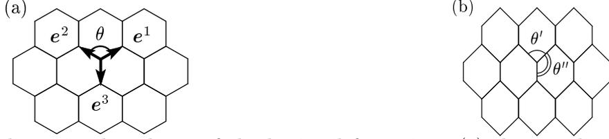
Fig. 1. Two dimensional analogue of the lattice deformation: (a) the two dimensional regular diamond (honeycomb) lattice and (b) the distorted lattice with  $e^3$  direction specified ( $\theta'' > \theta > \theta'$ ).
