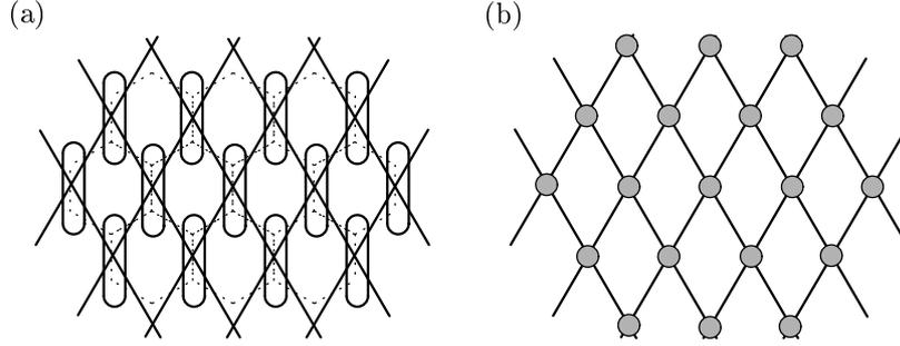
Fig. 3. (a) Translation symmetry of the honeycomb lattice. Unit cells consisting of  $L$ -node and  $R$ -node are encircled. (b) A deformed square (rhombus-like) lattice with the translation symmetry equivalent to that of the honeycomb lattice.
