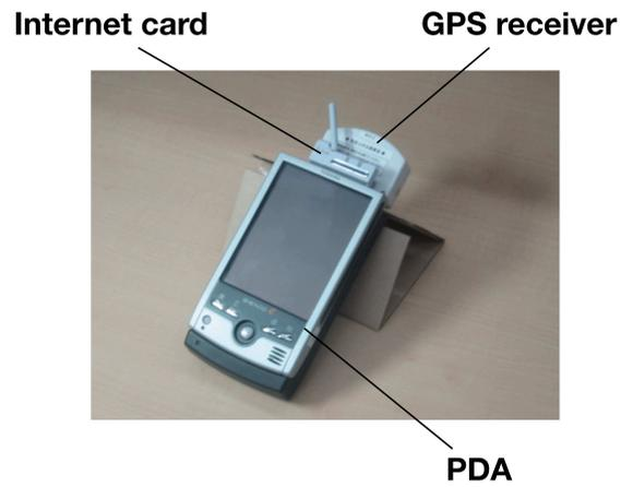
Figure 4.2: The client device
