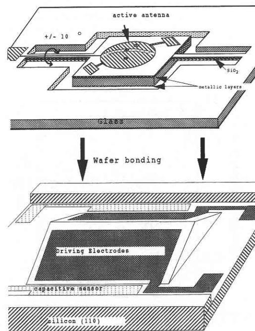
Fig.1 Functional diagram of a rotating antenna
