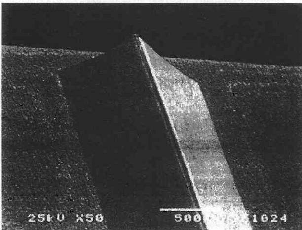
Fig.3 Triangular shape obtained by KOH etching
