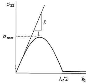
Fig. 2 Relation between Strain-like Quantity  $\tilde{\epsilon}_{22}$  and Restraining Stress
