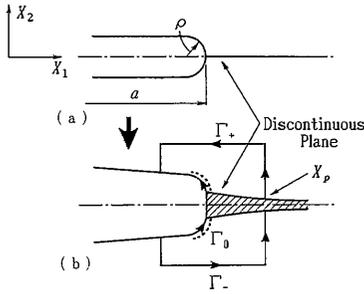
Fig. 1 Discontinuous Crack Model
