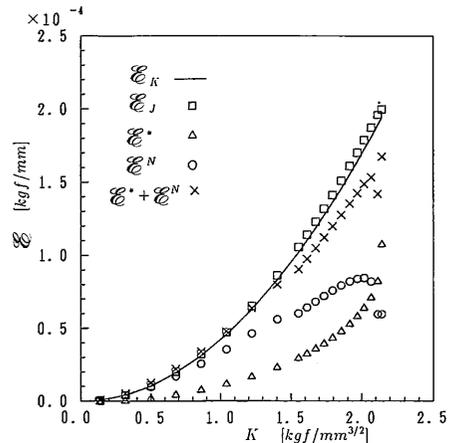
Fig. 5 CED Value with load ( $\rho=0.4 \times 10^{-6}$ mm)
