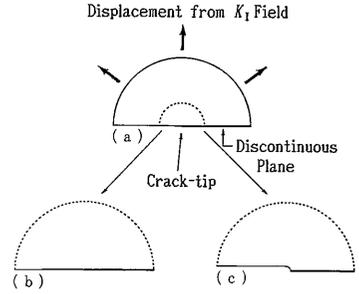
Fig. 3 Crack Model for Analyses
