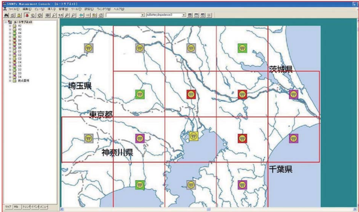
Fig. 2. Screen shot of Simple Network Management Protocol (SNMP) monitoring window. The colors of icons change from green to red through yellow and pink as the degree of the problem is increased.
