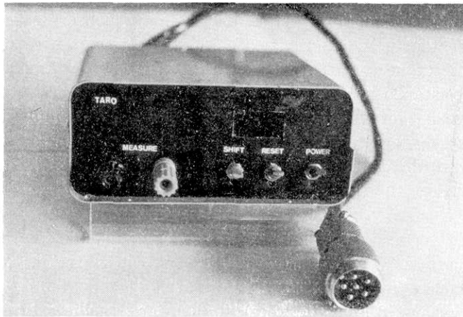
Fig. 5b. Picture of the controller. The two terminals shown on the left are used for measuring the resistance of the thermistors.
