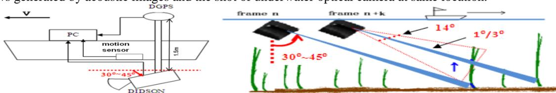
Fig. 2 Equipment setting & image of data collection of DIDSON system [3]
