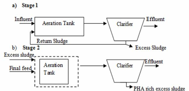
**Figure 1:** Two stage activated sludge process, a) stage 1: conventional activated sludge process; b) stage 2: FAREWEL process.
