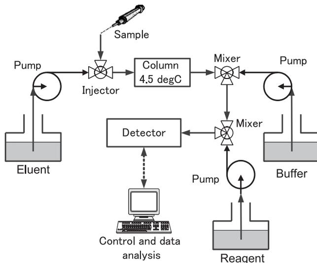
Fig. 4. Schematic diagram of an HPLC system.
