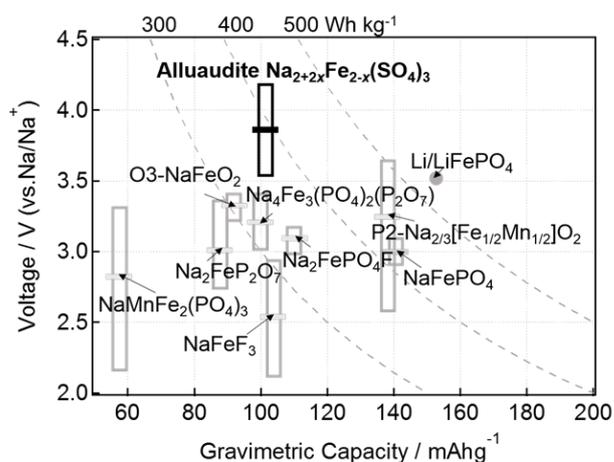
**Fig. 7** Overall comparison of the Fe-based cathode materials which can function as sodium sources in Na-ion battery system.
