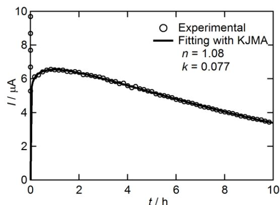
**Fig. 1** Chronoamperogram obtained for the  $\text{LiFePO}_4$  electrode under a 10 mV anodic step. The plots and line denote the experimental and simulating curves. Obtained Avrami exponent ( $n$ ) and rate constant of phase-boundary movement ( $k$ ) are presented.
