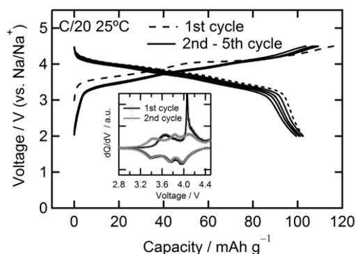
**Fig. 4** Voltage-capacity profiles of  $\text{Na}_{2+2x}\text{Fe}_{2-x}(\text{SO}_4)_3$  cathode cycled between 2.0 and 4.5 V at a rate of C/20 at  $25^\circ\text{C}$ . (Inset) The corresponding  $dQ/dV$  curves at the first two cycles.
