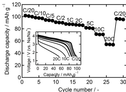
**Fig. 5** Capacity retention upon cycling up to 30 cycles under various rate of C/20 to 20C. (Inset) The corresponding discharge curves of  $\text{Na}_{2+2x}\text{Fe}_{2-x}(\text{SO}_4)_3$  as a function of rate.
