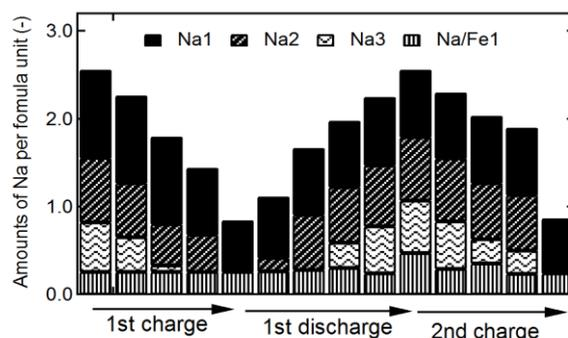
**Fig. 6** Amounts of sodium per formula unit in Na<sub>2+2x</sub>Fe<sub>2-x</sub>(SO<sub>4</sub>)<sub>3</sub> during the charge/ discharge processes.
