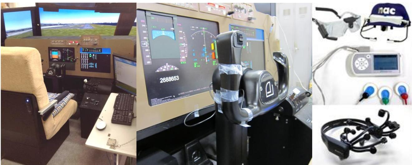
Fig. 4. Simulator of the Suzuki-Tsuchiya laboratory at The University of Tokyo. Left: overview. Middle: Sternberg 7 digits secondary task and response switches (Yellow & Orange) attached to the control column. Part of the primary flight display is covered for experiment’s primary task purposes. Right: Eye mark camera, Portable ECG device, and brainwave measurement headset.
