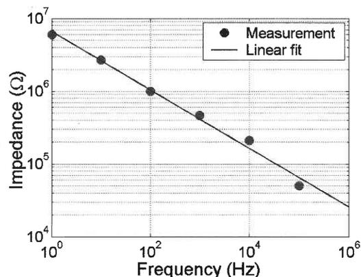
Figure 4 Measured impedance of microelectrodes with liposome solution versus frequency. At 300 kHz, it is about 40 k $\Omega$  which is compatible with the specifications of our power source.
