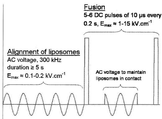
Figure 5 Voltage waveform for the electrofusion of liposomes.
