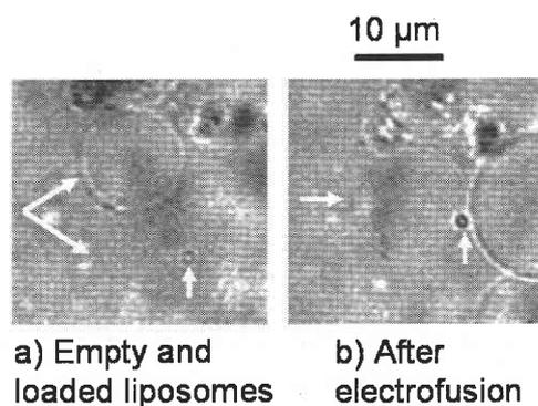
Figure 9 0.32 $\mu$ m microbeads transfer into an empty liposome by electrofusion with bulk electrodes.
