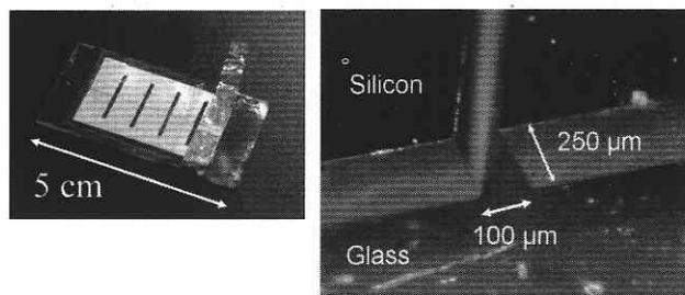
Figure 3 Photograph of the microfluidic device and close-up view of the high aspect-ratio silicon microelectrodes.
