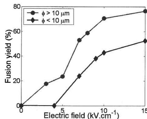
Figure 7 Experimental fusion yield as a function of the applied electric field for liposome diameters  $\phi$  larger and smaller than 10μm.
