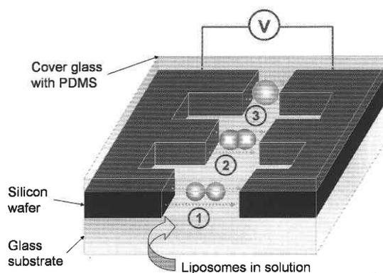
Figure 1 Schematic view of the device and protocol to fuse liposomes. Various gaps of electrodes have been designed. 1) Liposomes are aligned along the electric field lines by AC voltage. 2) DC pulses inducing high electric field perform the breakdown of membranes. 3) These membranes reconnect to form a hybrid vesicle.
