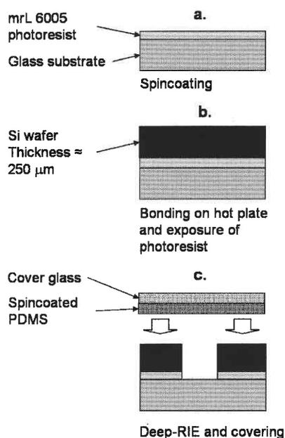
Figure 2 Fabrication process of the microelectrodes.
