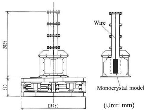
図2 Drawing of experimental model
