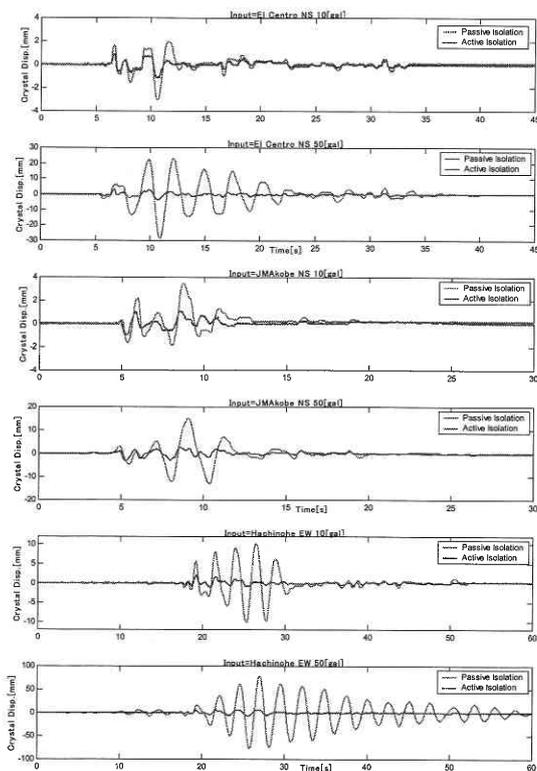
図 10 Time histories of displacement of crystal model
