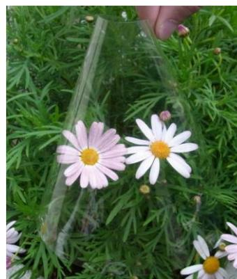
**Fig. 1.** Appearance of a cellulose film prepared from the NaOH/urea solution.
