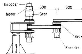
Fig. 1. Two-degree-of-freedom manipulator.
