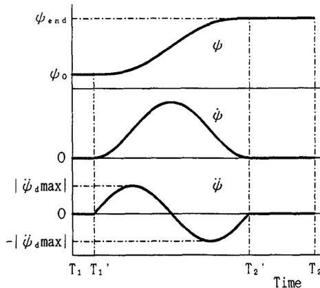
Fig. 3. Desired trajectory of the passive joint.
