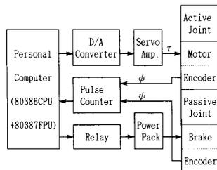
Fig. 5. Configuration of the control system.
