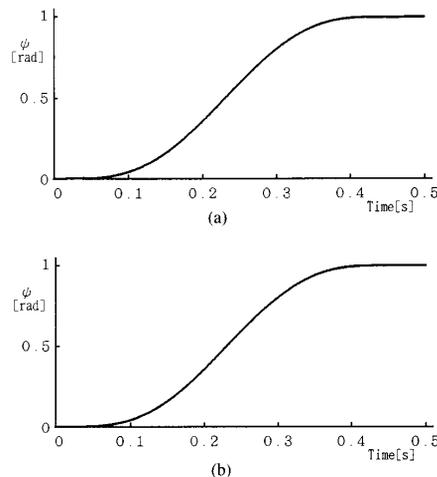
Fig. 7. Trajectory tracking of the passive joint: (a) Experimental result; (b) desired trajectory.
