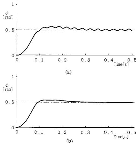
Fig. 6. Step response of the passive joint: (a) Experimental result by feedback (5); (b) experimental result by feedback (8).
