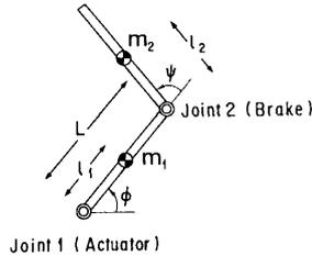
Fig. 2. Model of the manipulator.
