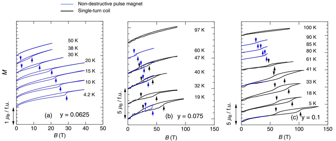
FIG. 2. Magnetization curves of  $(\text{Pr}_{1-y}\text{Y}_y)_{0.7}\text{Ca}_{0.3}\text{CoO}_3$  for (a)  $y = 0.0625$ , (b)  $0.075$ , and (c)  $0.1$ , measured at various temperatures using the induction method.
