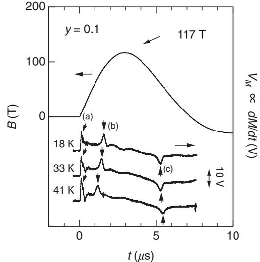
FIG. 1. Representative data of the induction voltage of the magnetization of  $(\text{Pr}_{1-y}\text{Y}_y)_{0.7}\text{Ca}_{0.3}\text{CoO}_3$  ( $y = 0.1$ ) and the pulsed magnetic field generated using the horizontal single-turn coils.
