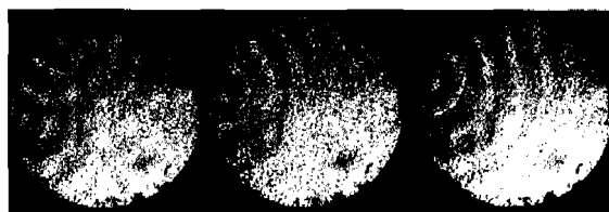
Fig. 5 Control of conduction-convection transition by magnetic fields. Left: onset of convection without the field, Center: suppression of convection by applying the field, Right: recovery of convection by removing the field
