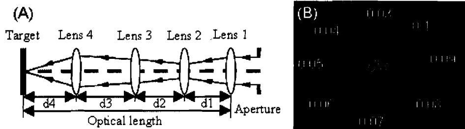
Figure 2: A schematic illustration of the optical system (A) and the profiles of laser spots on the target (B).
