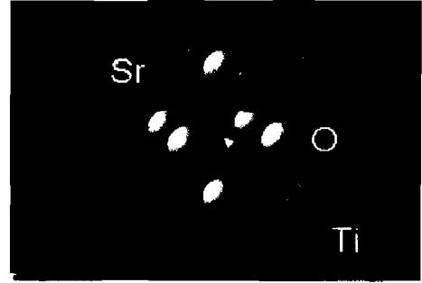
Figure 1: Atomic model of  $\text{SrTiO}_3$ . Ti atom is at the cube center surrounded by O atoms octahedrally and Sr atoms at the cube corners.
