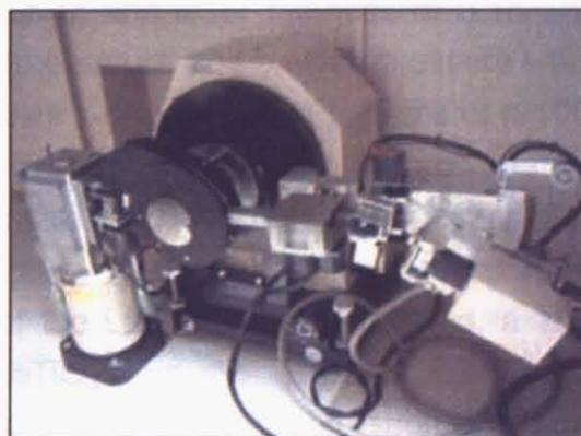
Fig.2-3-3-2 X-ray diffractometer
