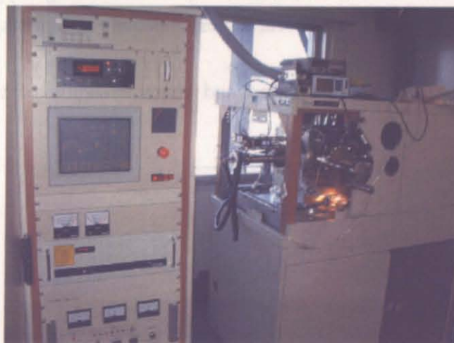
Figure 3.4 Photograph of the Ar ion milling machine.
