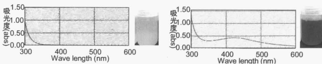
Fig. 8 Absorption spectrum of solution without bubbles and an image of the solution after ultrasonic irradiation. (Left: without microbubbles, Right: with microbubbles.)
