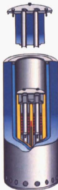
Fig.2.4 Internal structure of C80
