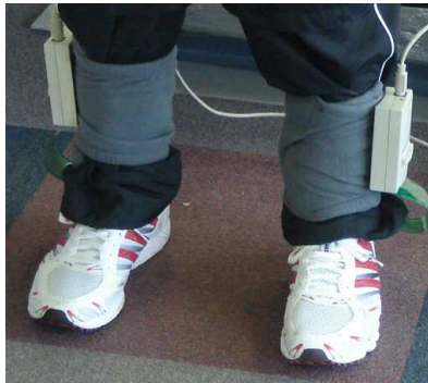
Figure 4-5: Signal processing units placed laterally at lower leg.
