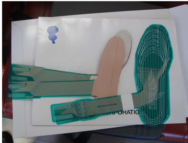
Figure 4-2: Sensors before (right) and after (left) preparation (Tekscan F-scan Lite System, cell model: 3000, distributed in Japan by Nitta Corporation).
