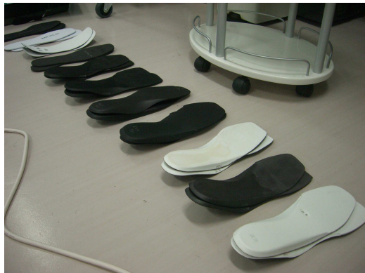
Figure 4-11: Some of the insoles used during experiment. From left to right: flat insoles (4 pairs) and conform insoles (7 pairs).
