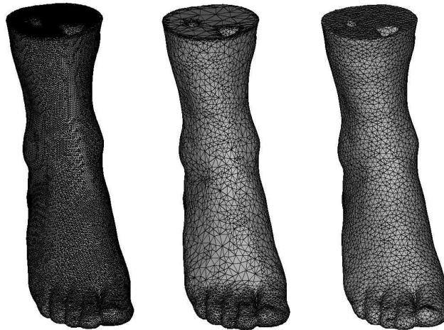
Figure 3-15: Example of the mesh reduction and smoothing for the soft tissues. Starting from the left: 1200 004 elements, 24880 elements, and 20144 elements.
