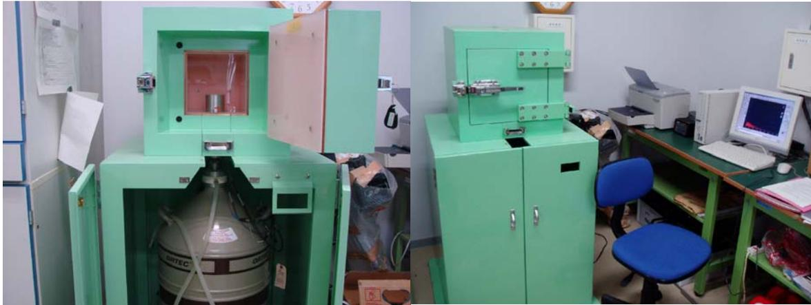
Plate 18 and 19: EG & G ORTEC GAMMA-X® HPGe, <sup>210</sup>Pb and <sup>137</sup>Cs Sediment Dating
