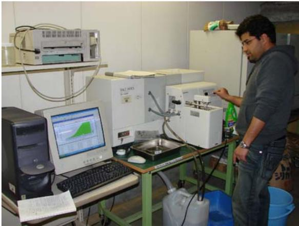
Plate 14: Laser Diffraction Particle Size Analysis
