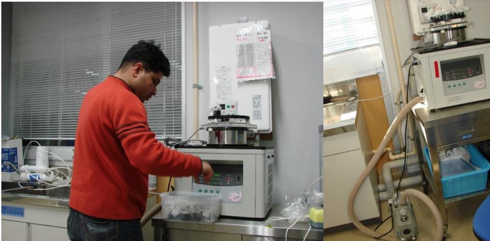
Plate 16: Freeze Drying of Sediment Sample (EYELA FDU-1200)
