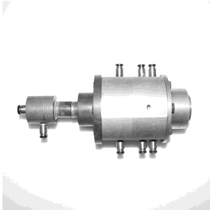
Figure 2.12: Arc heater made in Tokyo University
