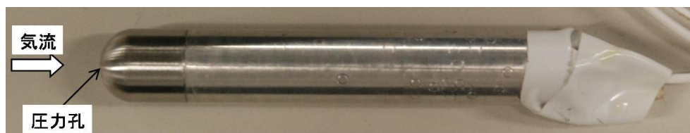
Figure 3.18 : Photograph of Pitot Tube
