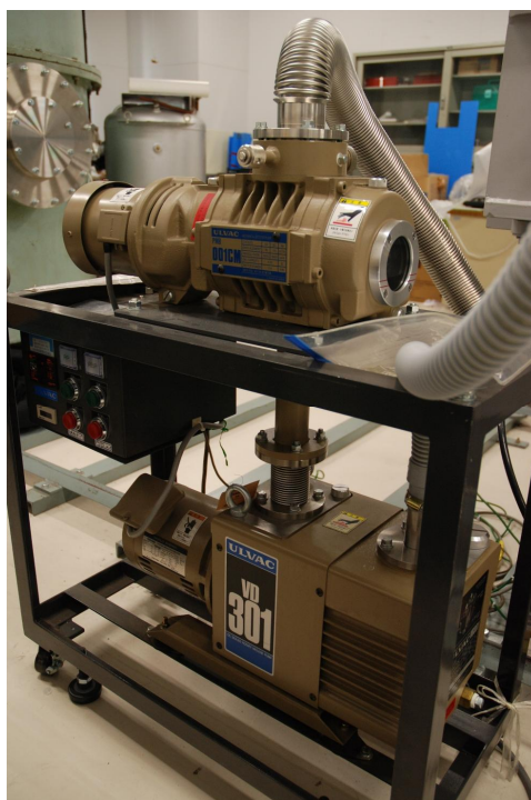
Figure 3.16 : Photograph of Mechanical Booster Pump
