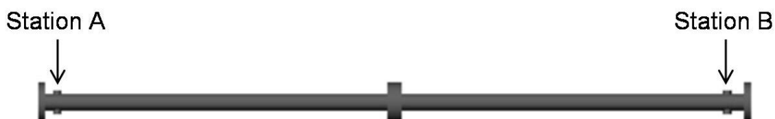
Figure 3.9 : The Location of Sensor Port
