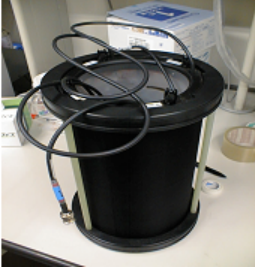
Fig.4.4 Birdcage RF coil (large type)
