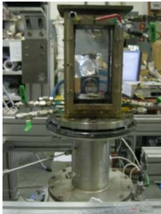
Fig. 3-2-2 square type combustion chamber for visualization
