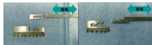
(a) previous type (b) improved type Fig. 2 Attachment between saw and linkage
