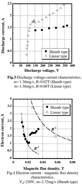
$V_d$ =250V, m=2.72mg/s (Sheath type  $V_d$ =250V, m=2.04mg/s (Linear type)
