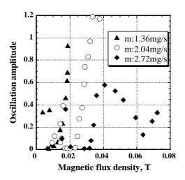
Fig.8 Relation between oscillation characteristics and magnetic flux density.
