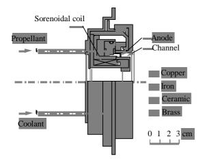
Fig.2 Cross-section of the linear type Hall accelerator.
