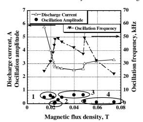
Fig. 5 Relation between oscillation characteristics and magnetic flux density.
