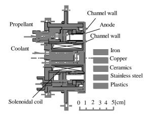
Fig.1 Cross-section of the sheath type Hall accelerator.
