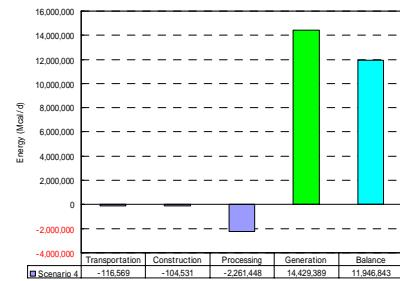
**Fig. 17.** Total Energy for each disposal process in Scenario 4.
