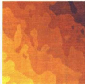
Figure 5.1. 1x1 μm<sup>2</sup> topography of an annealed Nb-doped SrTiO<sub>3</sub> substrate. 900° C for 1 hour in air
