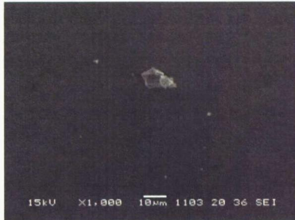
Figure 2.8 SEM image of particles in a  $\text{DyScO}_3$  thin film grown on a  $\text{SrTiO}_3$  substrate
