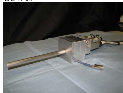
Fig. 1 Wedge prism 3D endoscope
