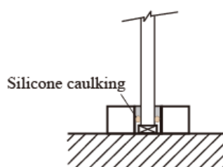
Fig. 5.15 Schematic representation of glass mounting using silicone caulking.
